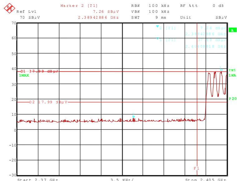
113324\_74.wmf: Radiated band-edge compliance, upper band edge, hopping off:
