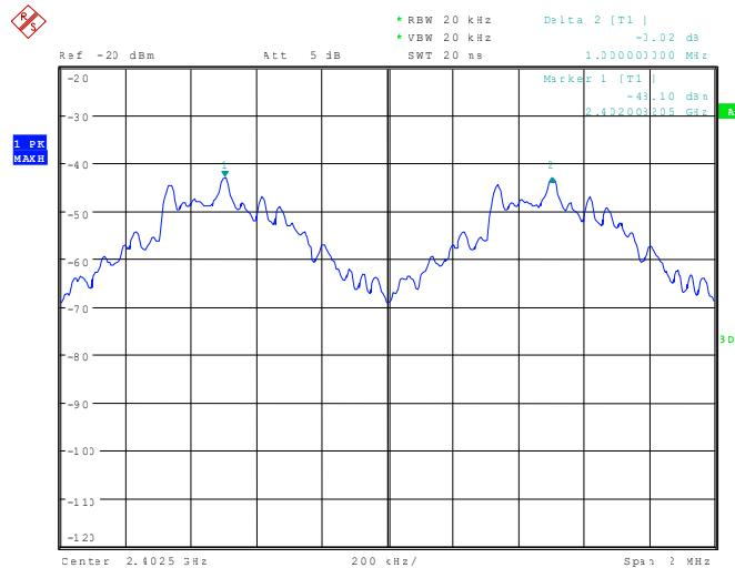
113324\_86.wmf: Channel separation at the middle of the assigned frequency band:
