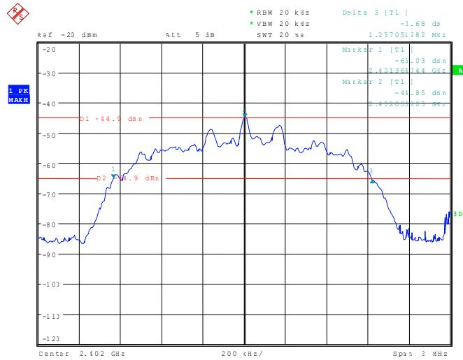
113324\_80.wmf: 20 dB bandwidth at the middle of the assigned frequency band:
