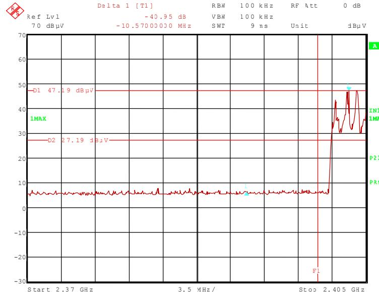
113324\_92.wmf: Radiated band-edge compliance, colocation, upper band edge, operation mode 5:
