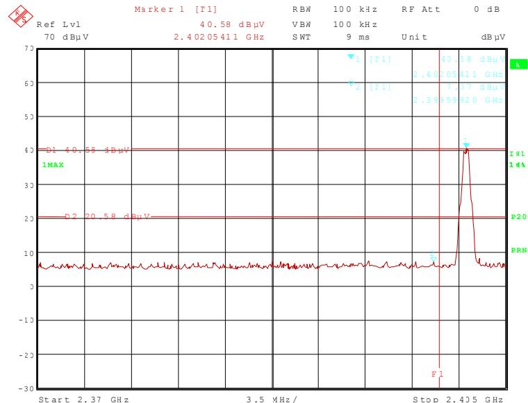
113324\_73.wmf: Radiated band-edge compliance, lower band edge, hopping on:
