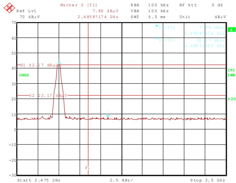
113324\_75.wmf: Radiated band-edge compliance, upper band edge, hopping on:
