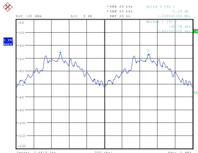
113324\_42.wmf: Channel separation at the upper end of the assigned frequency band:
