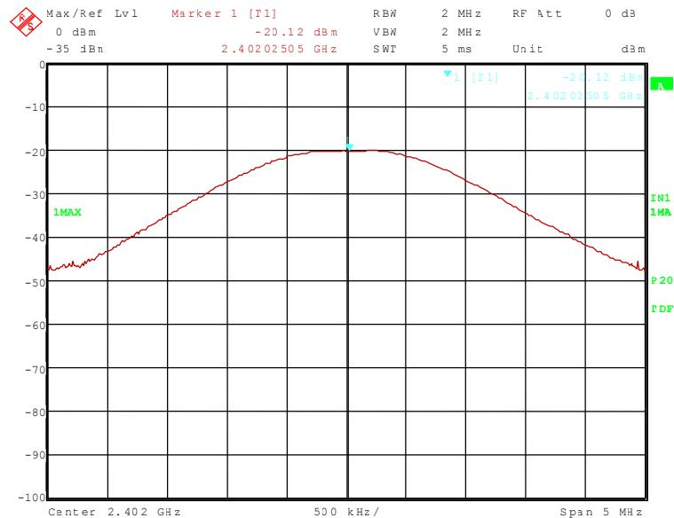
113324\_77.wmf: Maximum peak output power at the middle of the assigned frequency band (operation mode 2):
