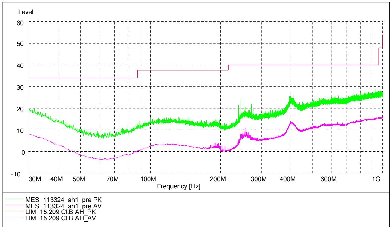
In this case it was not necessary to carry out subsequent measurements because at no frequency was a value above the Qualify limit curve during the preliminary measurements.
