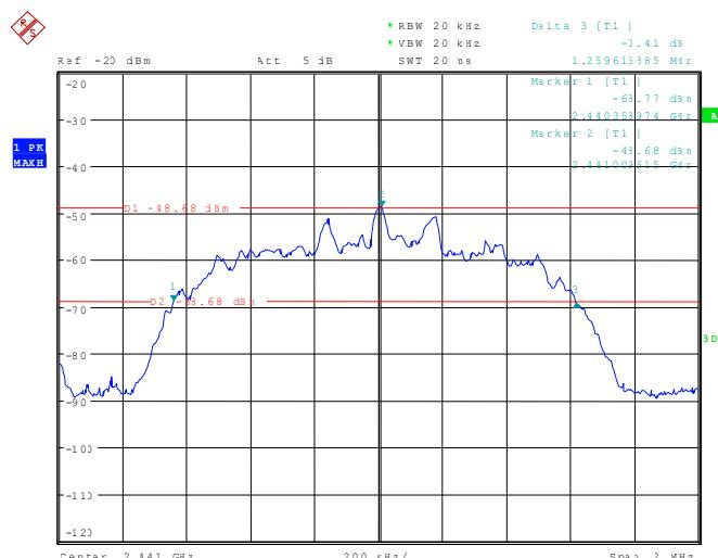
113324\_81.wmf: 20 dB bandwidth at the upper end of the assigned frequency band:
