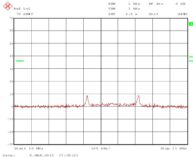
The centre frequency of the transmitter was found at 10.57 MHz. It had to be measured on the outdoor test site. The results are shown in clause 5.7.3.2.
