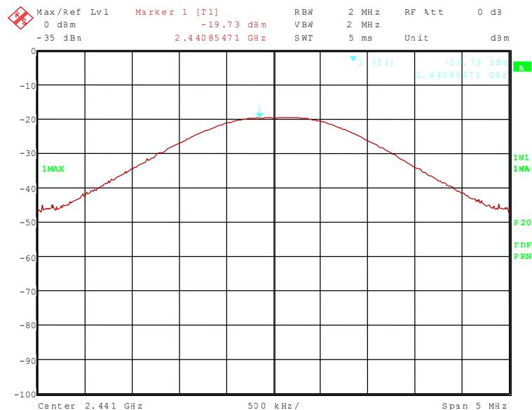
113324\_78-1.wmf: Maximum peak output power at the upper end of the assigned frequency band (operation mode 3):
