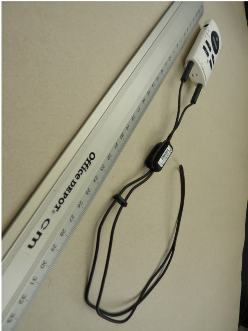
113324_34: Multistreamer (with connected loop antenna and ferrite core)
