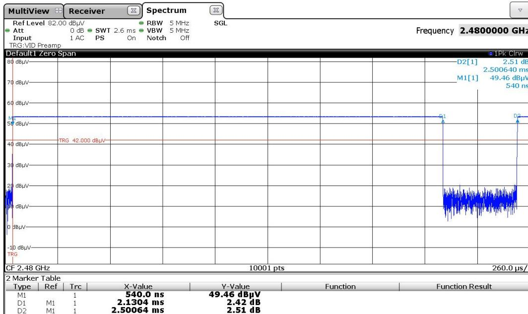
Since only one modulation is tested, the calculation is only performed for the worst case, namely the DH5 mode with GFSK modulation.
