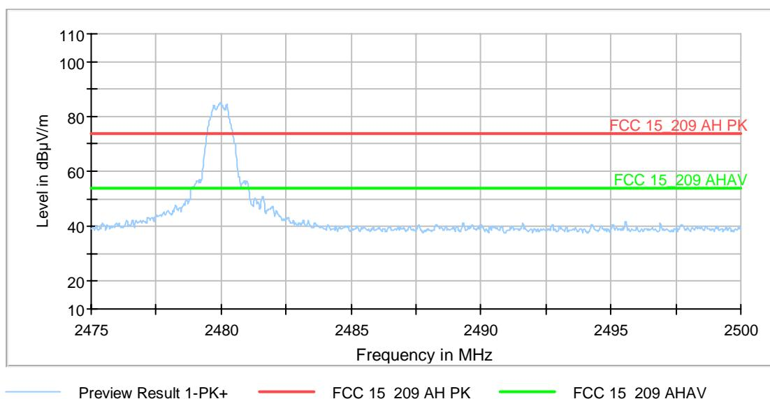
**Transmitter operates at the lower end of the assigned frequency band (operation mode 1 GFSK)**
