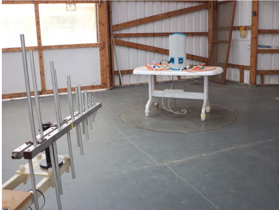
Photograph No.2 Setup for spurious emission measurements at the OATS
