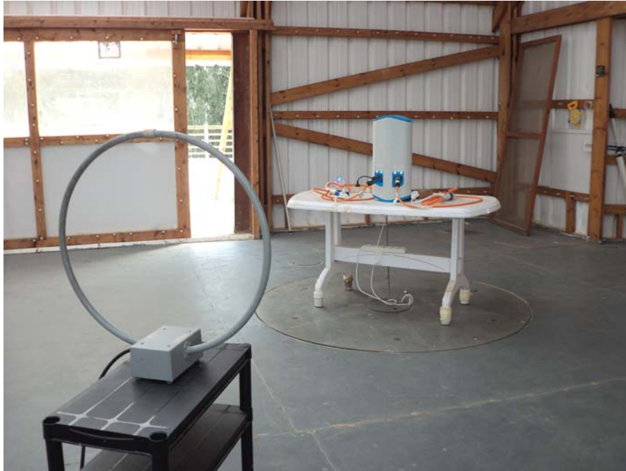
Photograph No.1 Setup for in-band emission and occupied bandwidth measurements at the OATS
