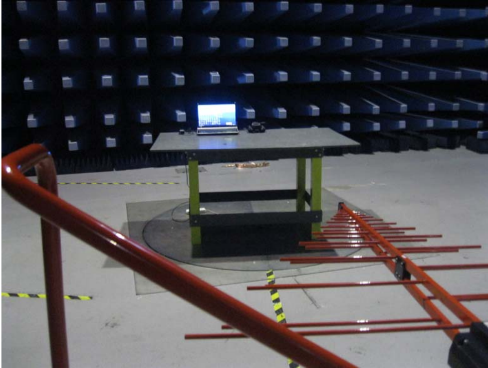
Radiated Emissions Setup Front View
