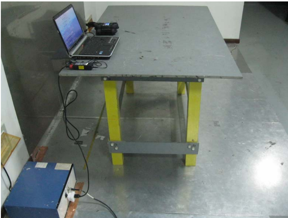
Conducted Emissions Setup Side View
