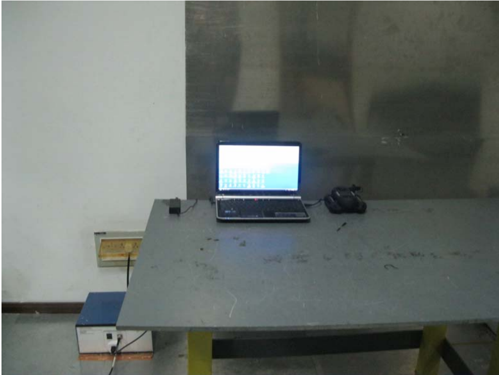
Conducted Emissions Setup Front View
