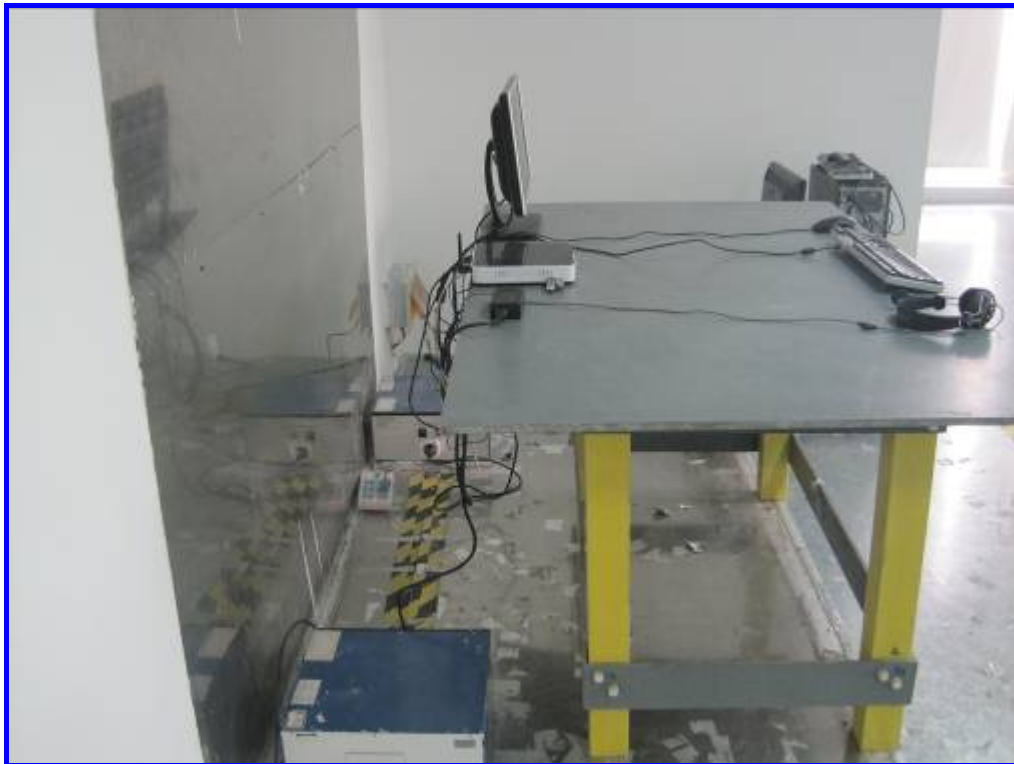
Side View of Conducted Emission Test Setup
