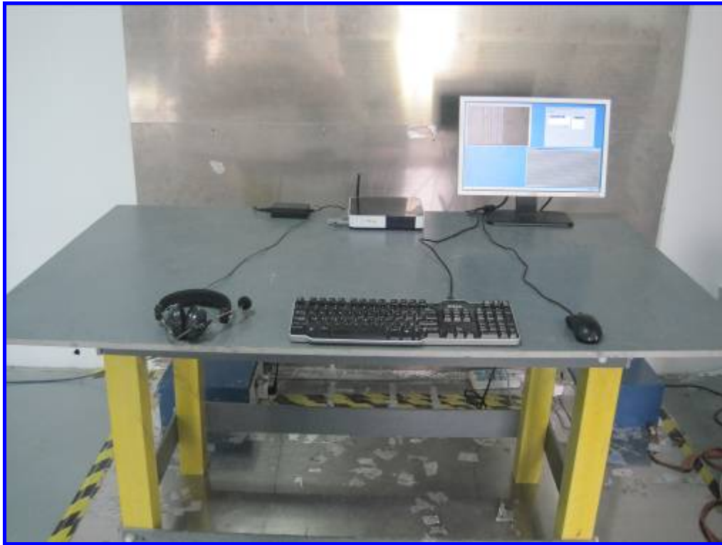
Front View of Conducted Emission Test Setup
