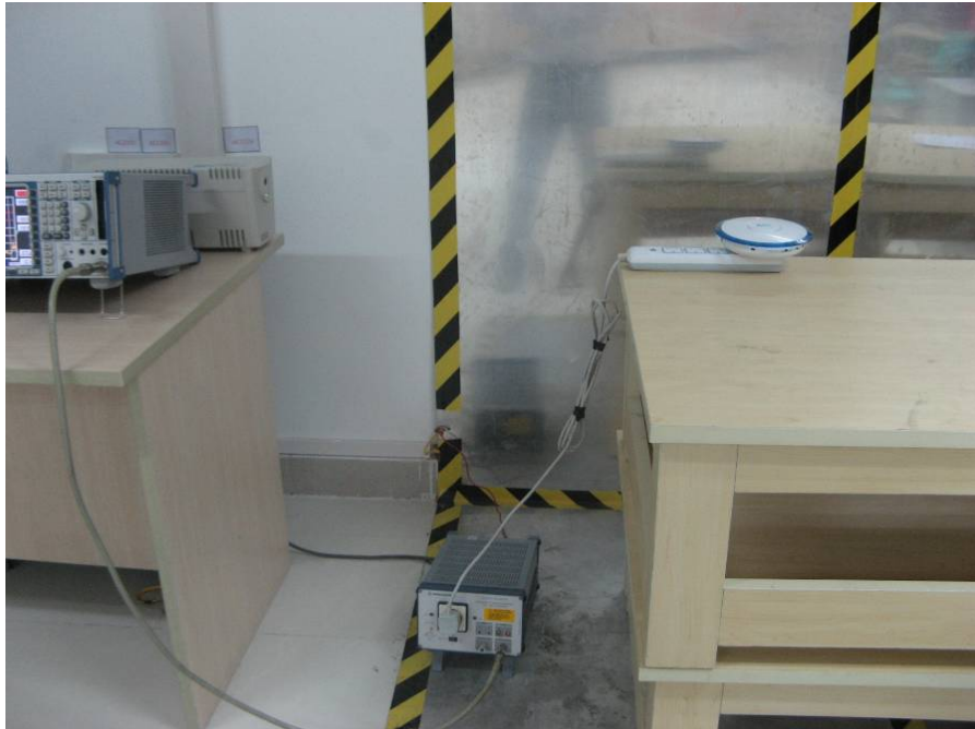
RADIATED EMISSION TEST SETUP
