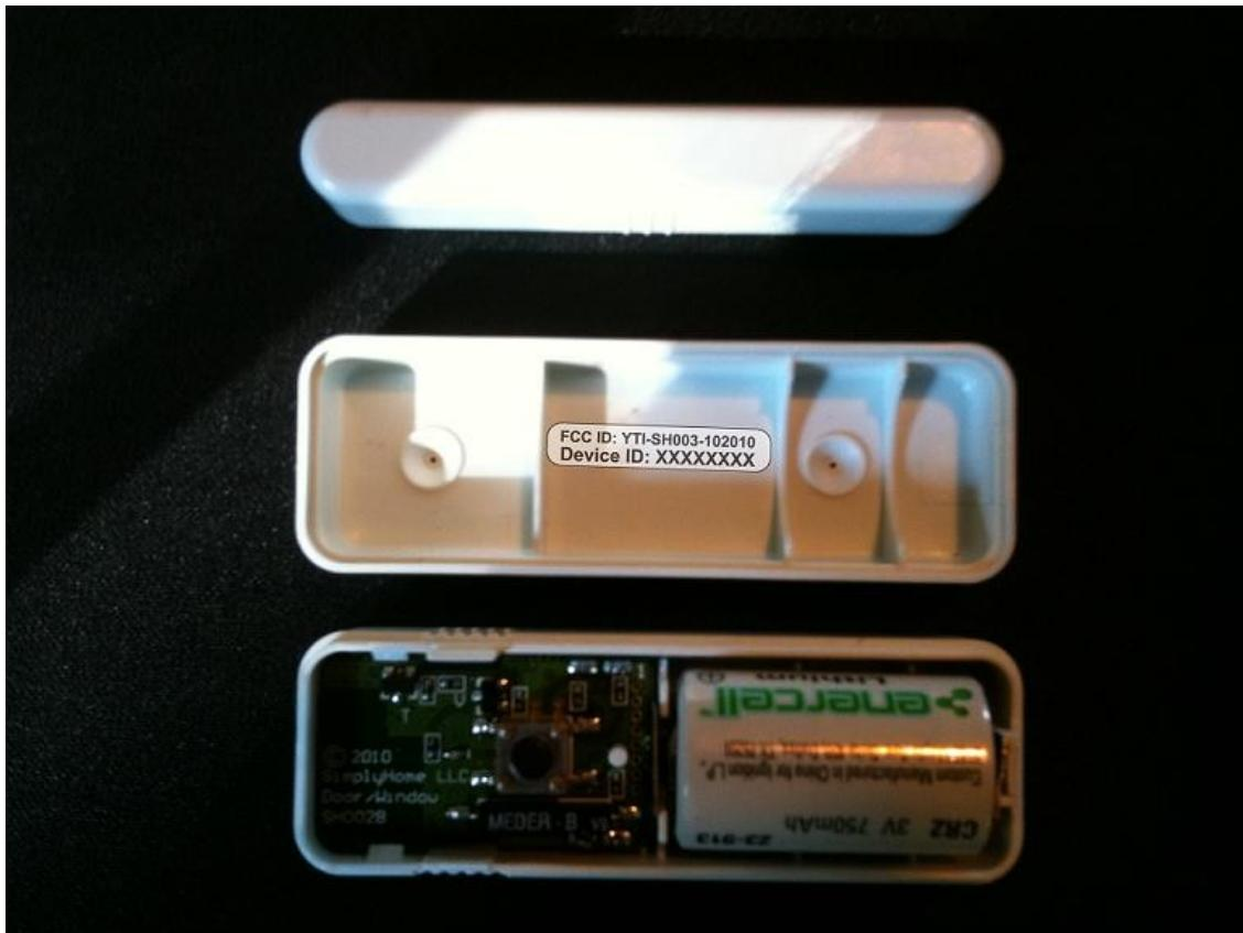
The consumer packaging for the Door/Window Contact includes the battery as a separate item. The FCC Identifier is visible to the user when it is marketed and when the battery is installed.
