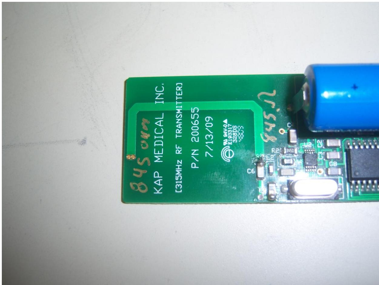
The Antenna is a trace on the circuit board. It is not possible for the user to replace the antenna or use an antenna other than the one provided. The circuit board is potted preventing the user from having access to the antenna or any other component.
