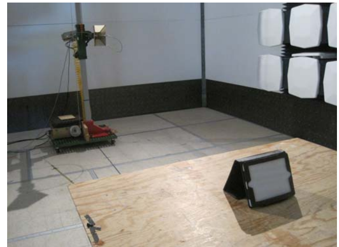
Radiated Emission (above 1GHz)- Rear View
