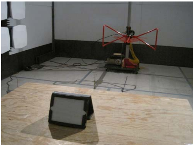
Radiated Emission (30MHz to 1GHz)- Rear View
