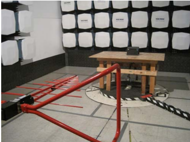
Radiated Emission (30MHz to 1GHz)- Front View
