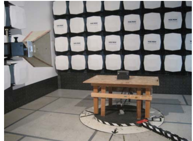
Radiated Emission (above 1GHz)- Front View
