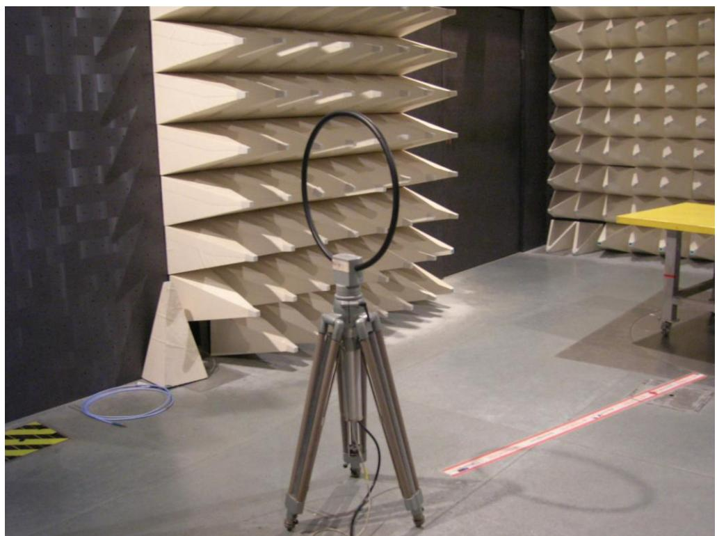
For radiated emissions 30MHz~1GHz
