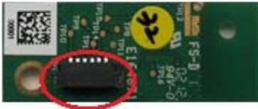
6-Pin Connection is standard USB2.0 specifications, could be applied to Microsoft Windows system the Notebook or Computer, need to refer to the motherboard of USB2.0 circuit configuration ◦
