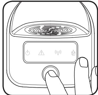
To test the Bed Shaker 520 or any Crossfire alarm, press and release the button on the front face of the unit.
