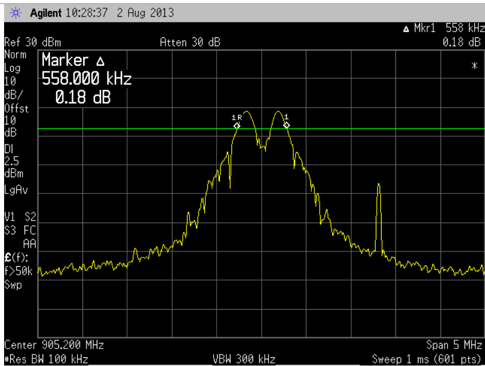
905.2 MHz: Observed 6 dB Bandwidth is 0.558 MHz
