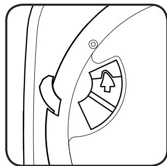
Activate your first alarm by moving the slide switch located on the back side of the alarm in the direction indicated by the arrow.
