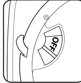
With the pin still pressed firmly in place, slide the switch in the direction indicated by the arrow in the drawing.
