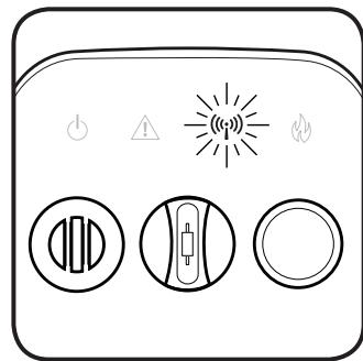
Activate your next alarm by moving its slide switch as shown above.
