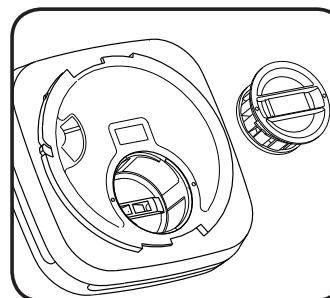
Carefully clean both the chamber **and** the empty alarm cavity with compressed air.
