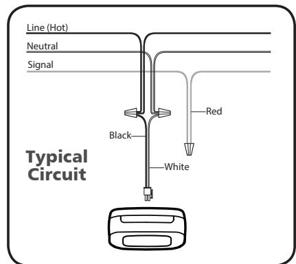
**With the AC power turned off**, connect the wire harness provided with the alarm.
