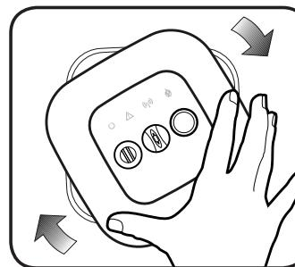
Re-install the smoke chamber into the cavity with a clockwise rotation. Align the dots on chamber and housing to ensure a proper fit.
