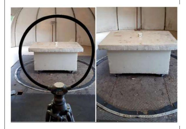
Photograph for Unwanted Emission in restricted frequency bands
