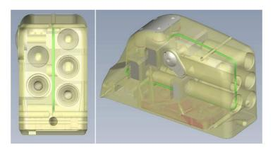
The DF-4 cavity diameter being bigger (6,35 mm), we had to route RF antenna wire around the DF-4 cavity. Please refer to the 2 pictures below (RF antenna highlighted in green in below 3D pictures).
