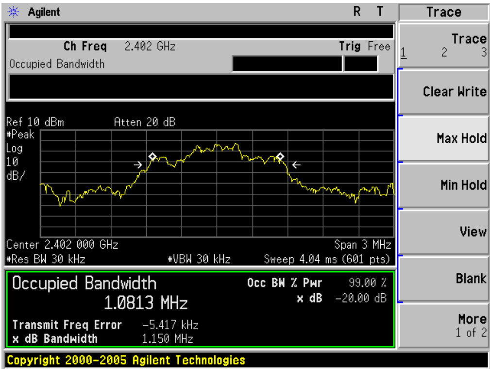
TEST PLOT OF BANDWIDTH FOR LOW CHANNEL
