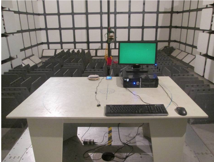
Radiated Emissions – Front View (Above 1 GHz)
