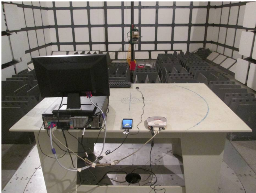
Radiated Emissions – Rear View (Above 1 GHz)
