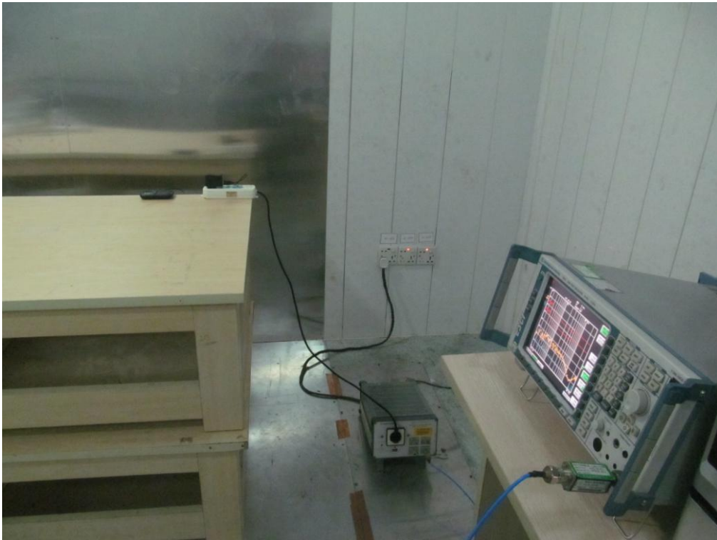
FCC RADIATED EMISSION TEST SETUP
