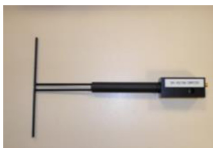
Figure 1 – Satimo COMOSAR Validation Dipole
