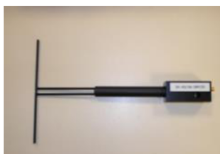
Figure 1 – Satimo COMOSAR Validation Dipole
