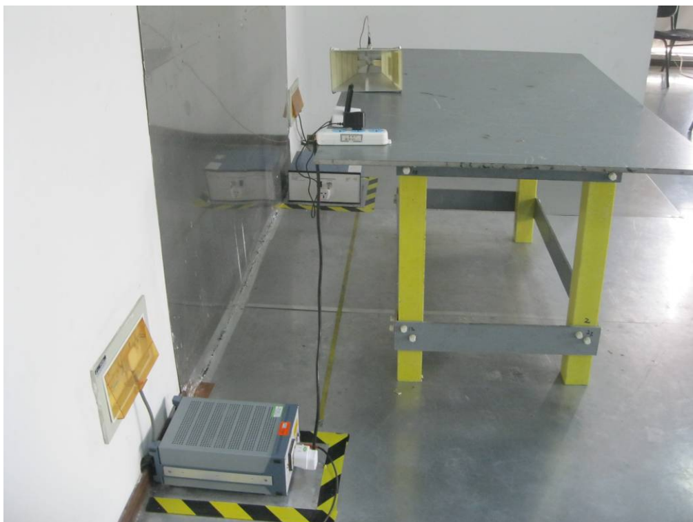
Conducted Emissions Test Setup Side View
