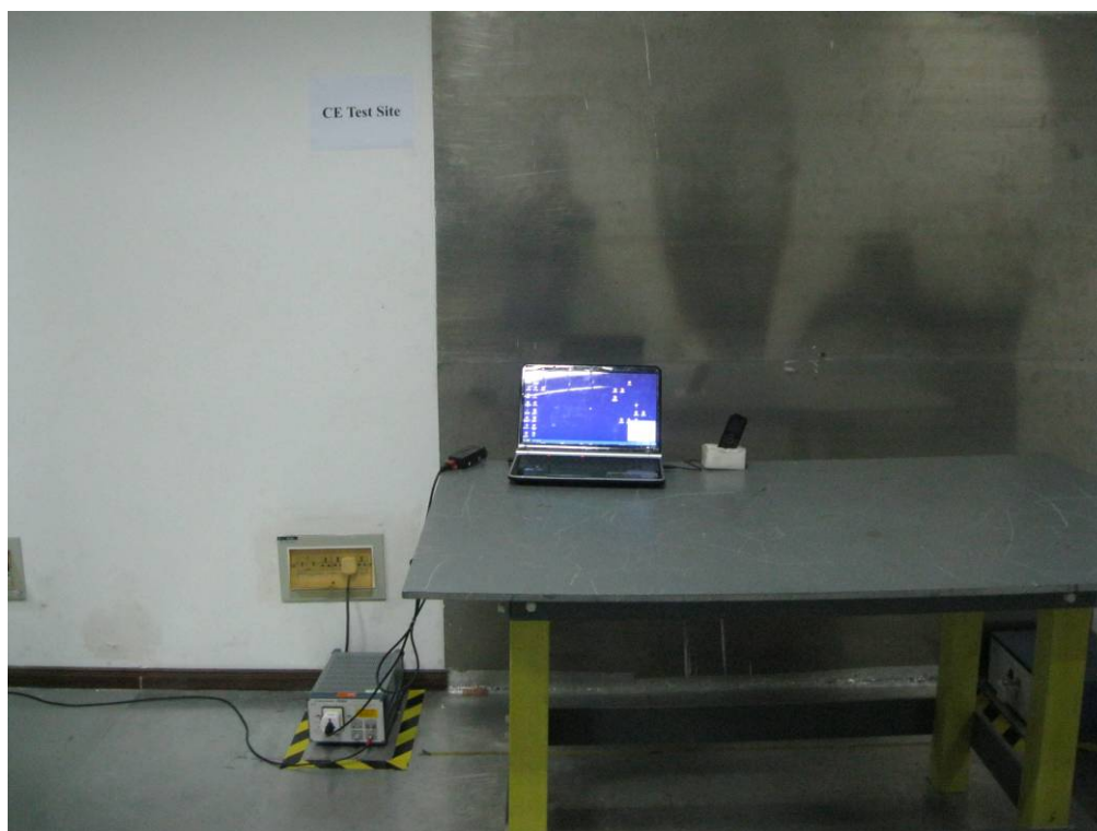
Conducted Emissions Test Setup Front View
