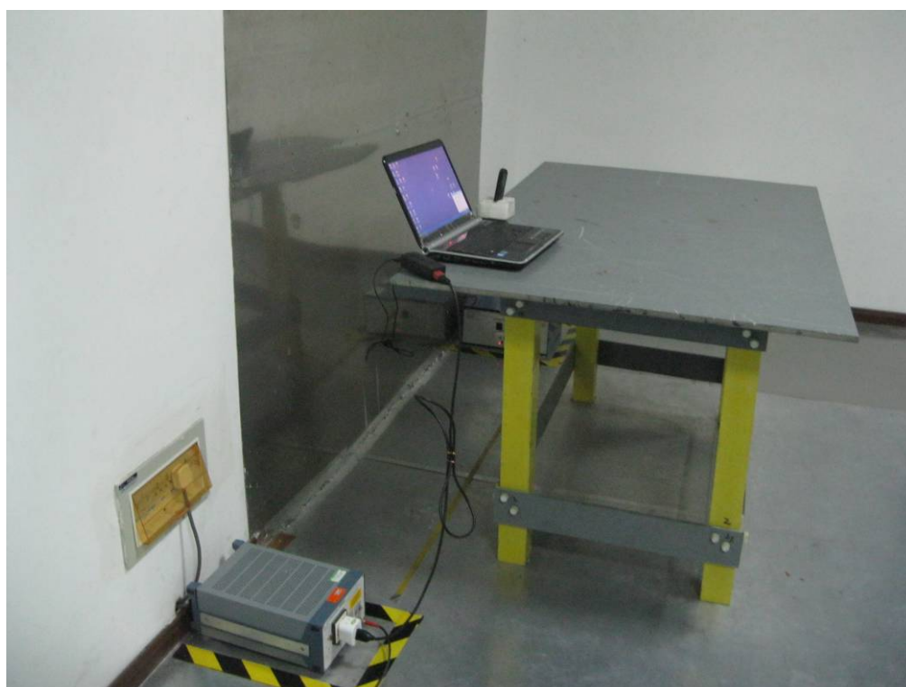
Conducted Emissions Test Setup Side View
