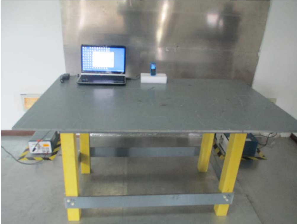
Conducted Emissions Test Setup Front View
