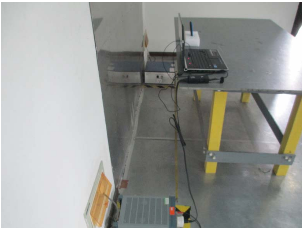
Conducted Emissions Test Setup Side View
