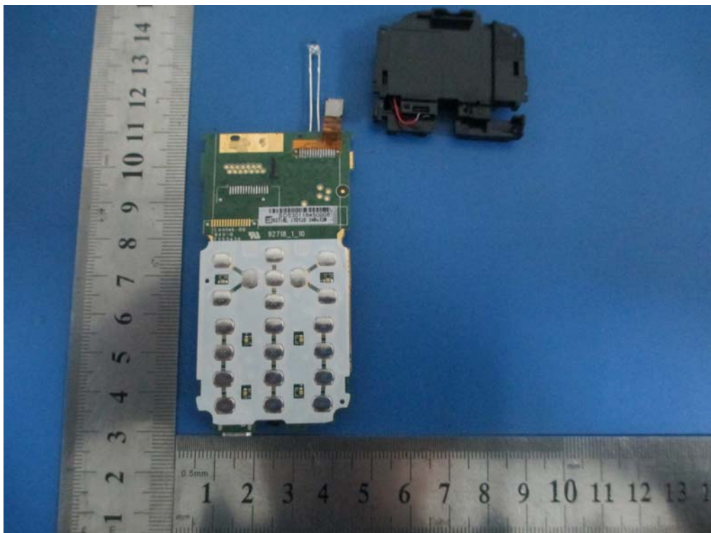
Uncover – Without Shielding Rear View
