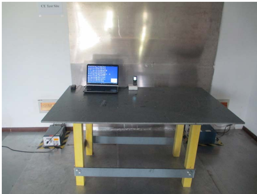
Conducted Emissions Test Setup Front View
