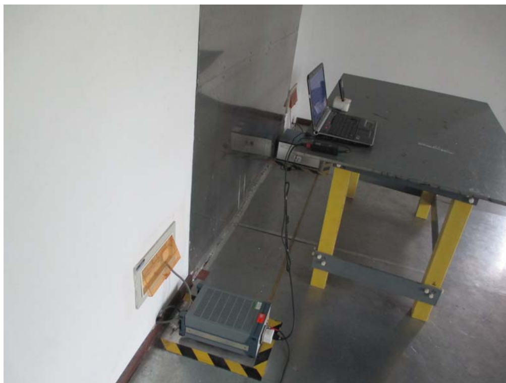
Conducted Emissions Test Setup Side View
