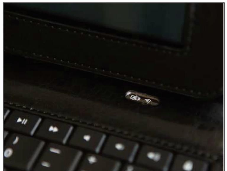
While the Rubata Keyboard is charging, the top left recharge light will illuminate.
