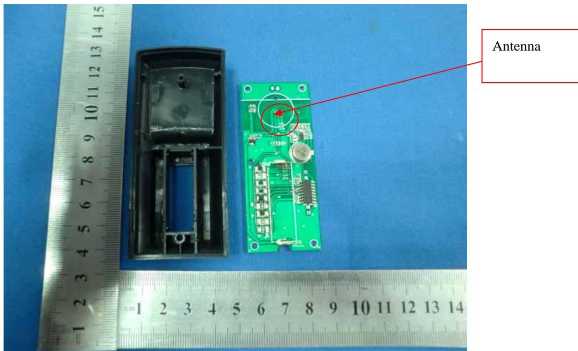
Internal Photo for model: FC-368M, FC-226, FC-468M, FC-328, FC-338
