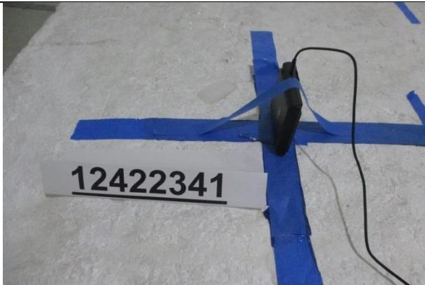
A photograph showing the same setup as the X-axis orientation, but from a different angle. The black device is mounted on the white card, which is secured to the surface with blue painter's tape in an X-shape. The device is connected by a black cable to an off-camera receiver.                                                                        |
