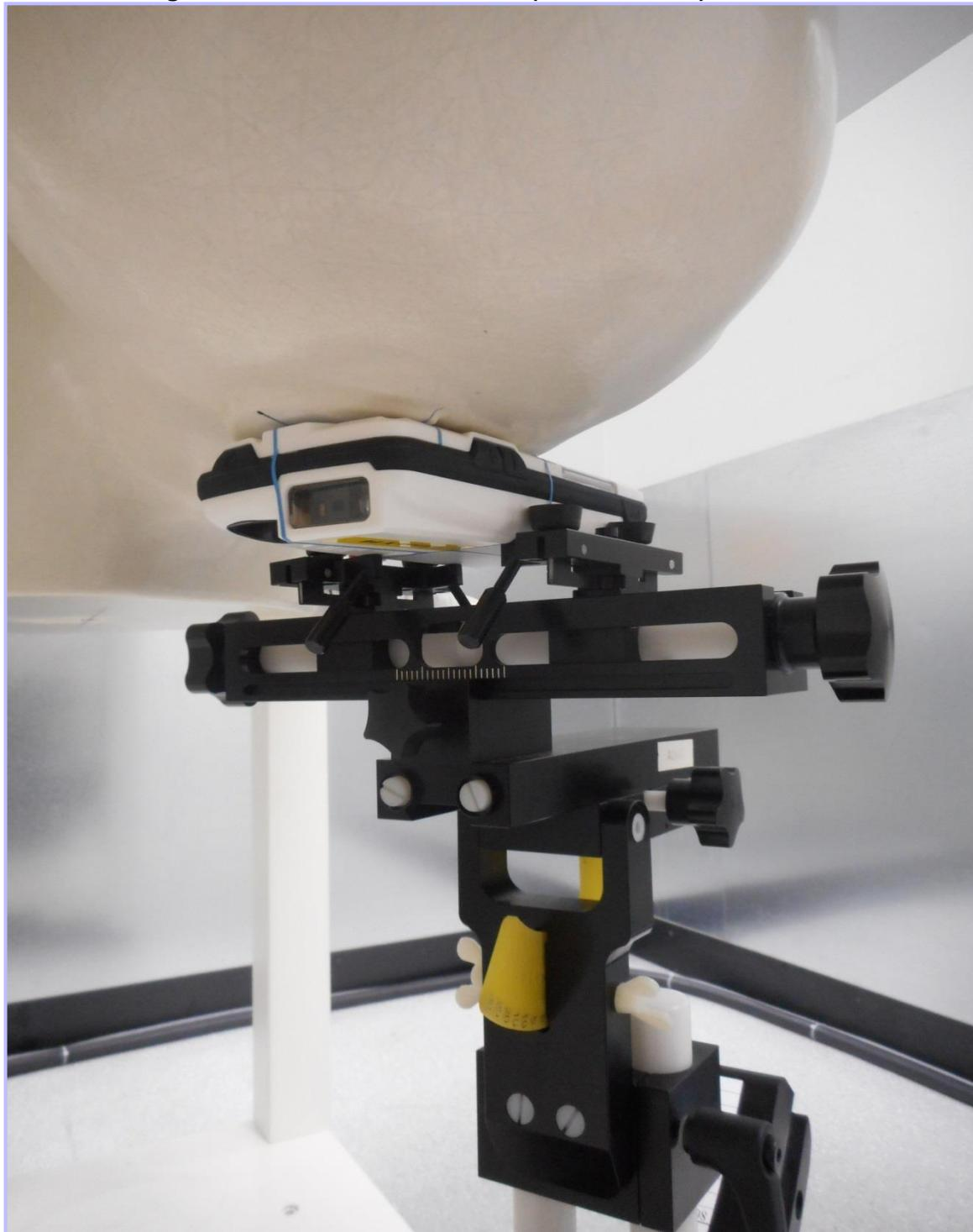
**008: Front of Host Device with Sleeve (InfineaX Case) Facing Phantom at 10mm Separation**
