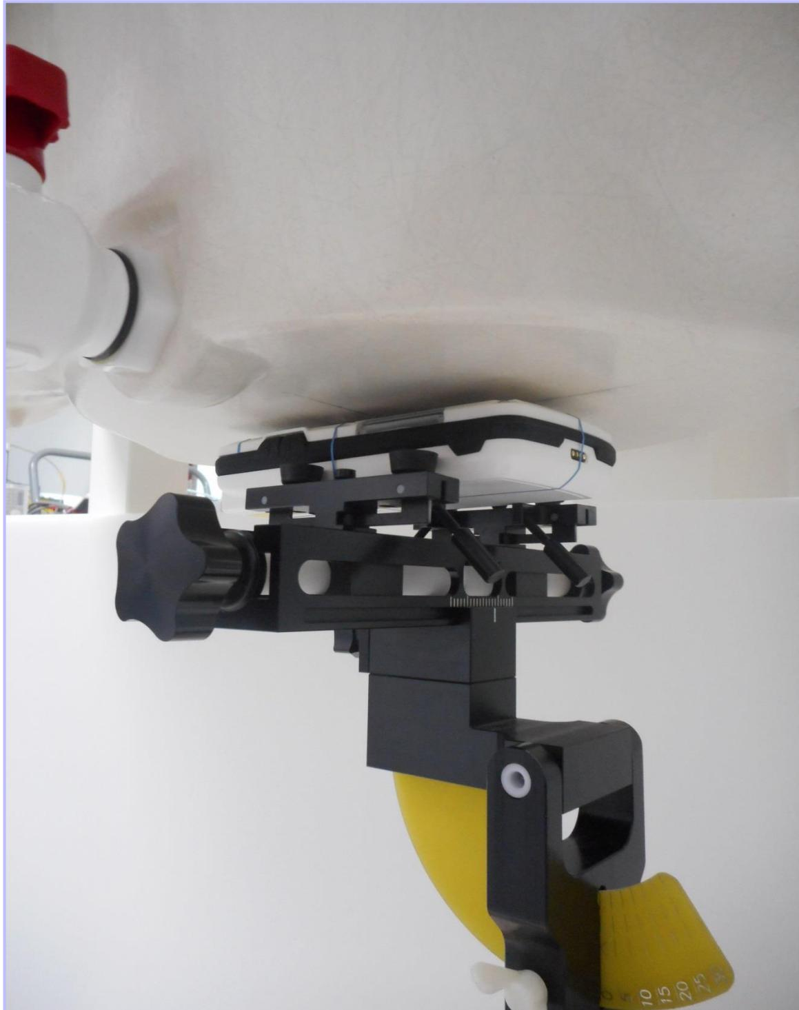
**009: Back of Host Device with Sleeve (InfineaX Case) Facing Phantom at 10mm Separation**
