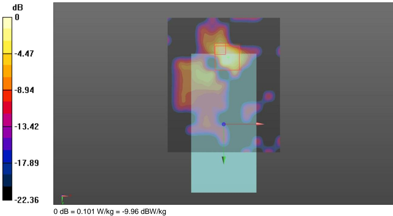
Communication System: UID 0, WLAN 802.11 (0); Frequency: 5320 MHz; Duty Cycle: 1:1
