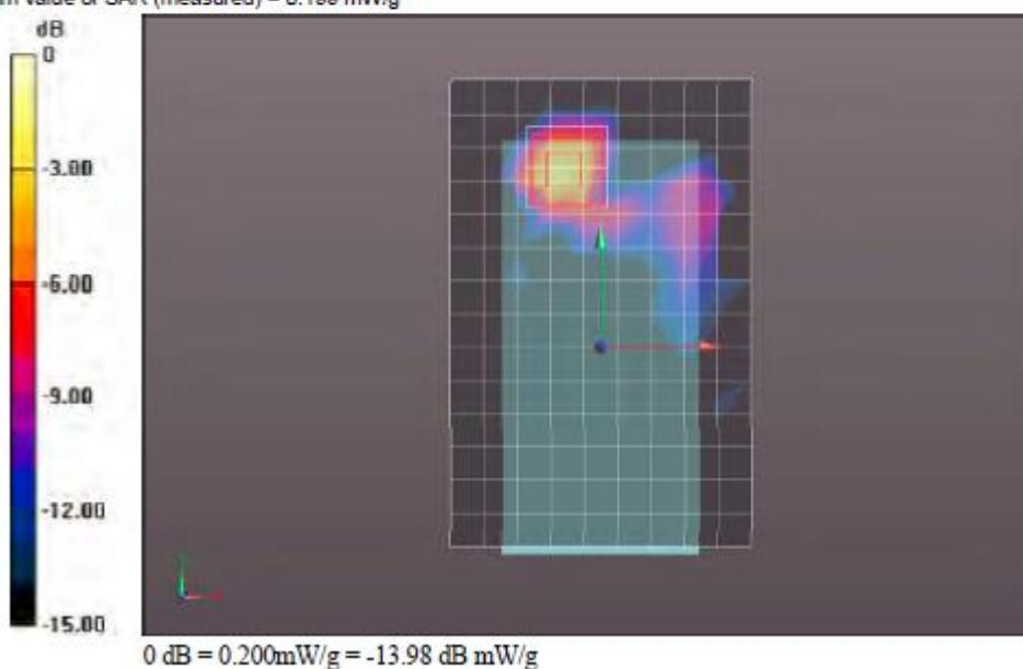
Front of EUT Wi-Fi 5.8 GHz CH149 - UL VS Ltd
