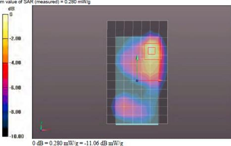
Touch Right of EUT Wi-Fi 5.3 GHz CH52 - UL VS Ltd
