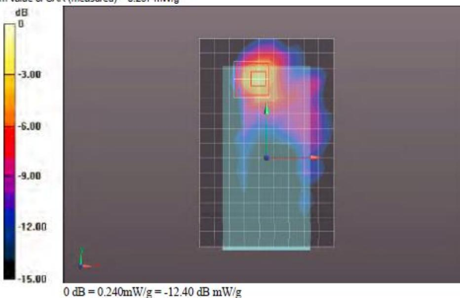
Front of EUT Wi-Fi 5.5 GHz CH116 - UL VS Ltd
