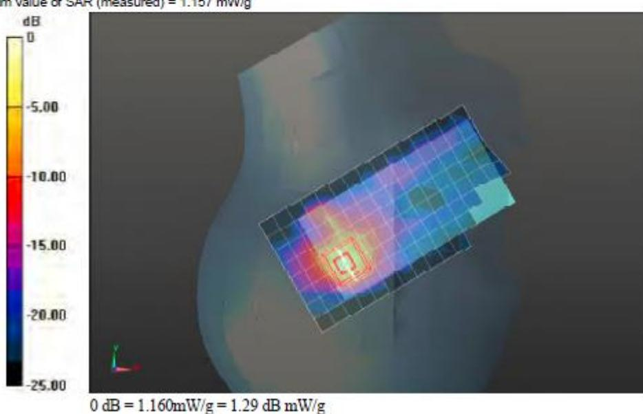
Touch Right of EUT Wi-Fi 5.5 GHz CH136 - UL VS Ltd
