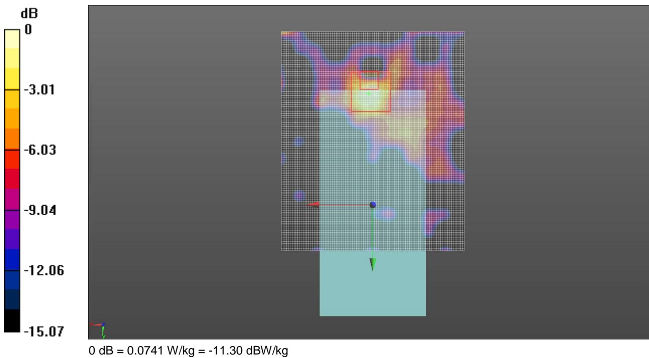
Communication System: UID 0, WLAN 802.11 (0); Frequency: 5580 MHz; Duty Cycle: 1:1
