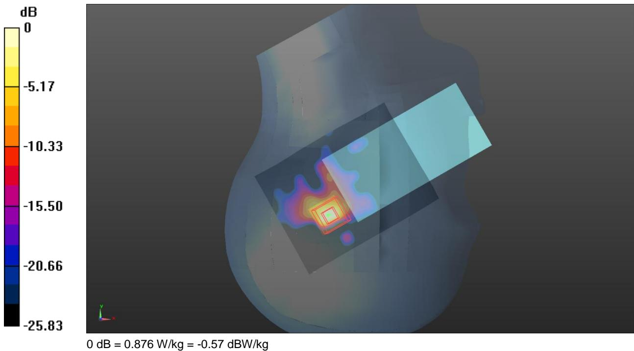
Communication System: UID 0, WLAN 802.11 (0); Frequency: 5260 MHz; Duty Cycle: 1:1
