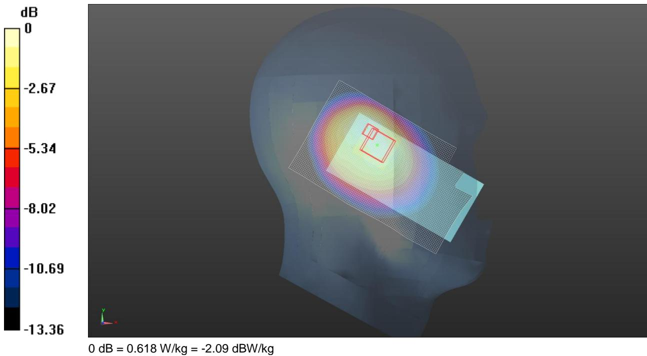
Communication System: UID 0, CDMA2000 (0); Frequency: 823.1 MHz; Duty Cycle: 1:1
