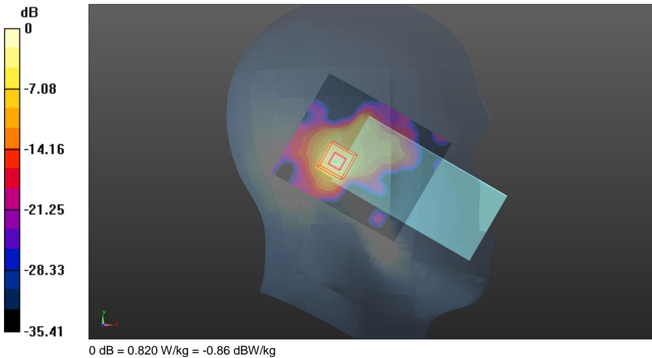
Communication System: UID 0, WLAN 802.11 (0); Frequency: 5240 MHz; Duty Cycle: 1:1
