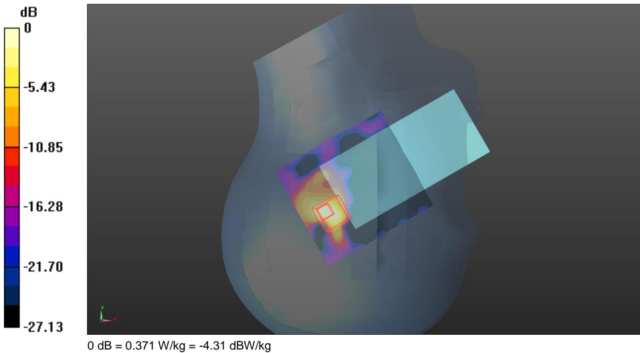
Communication System: UID 0, WLAN 802.11 (0); Frequency: 5680 MHz; Duty Cycle: 1:1
