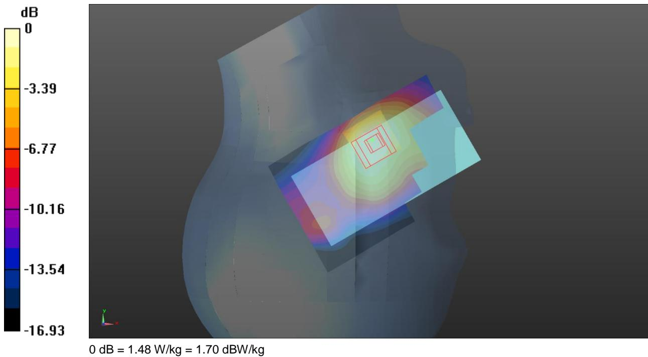
Communication System: UID 0, LTE - Band 4 / 20MHz Channel; Frequency: 1720 MHz; Duty Cycle: 1:1
