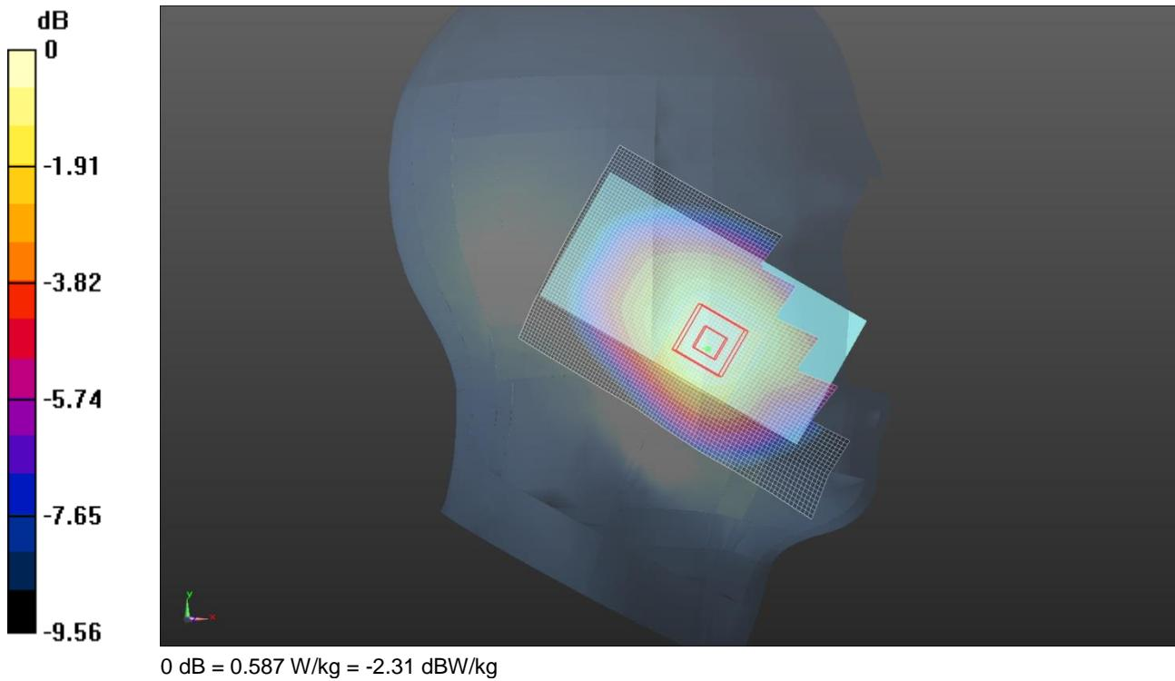
Communication System: UID 0, Generic GSM (0); Frequency: 836.6 MHz; Duty Cycle: 1:8.30042
