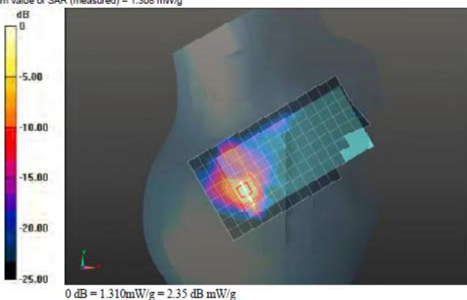
Front of EUT Wi-Fi 5.5 GHz CH124 - UL VS Ltd
