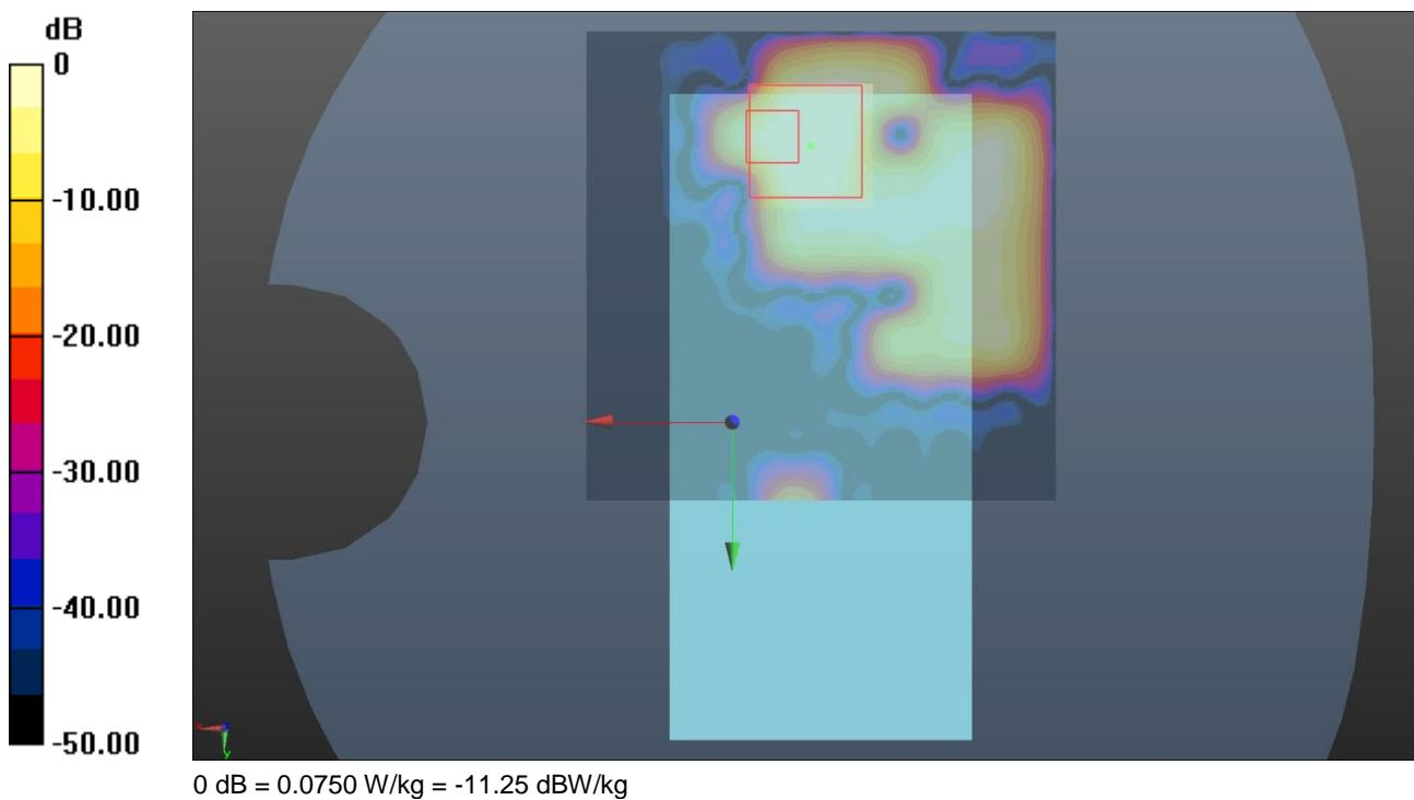
Communication System: UID 0, WLAN 802.11 (0); Frequency: 5745 MHz; Duty Cycle: 1:1
