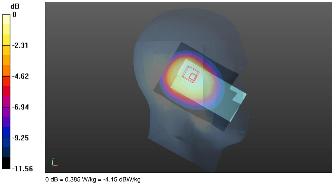
Communication System: UID 0, LTE - Band 13 / 10MHz Channel; Frequency: 782 MHz; Duty Cycle: 1:1
