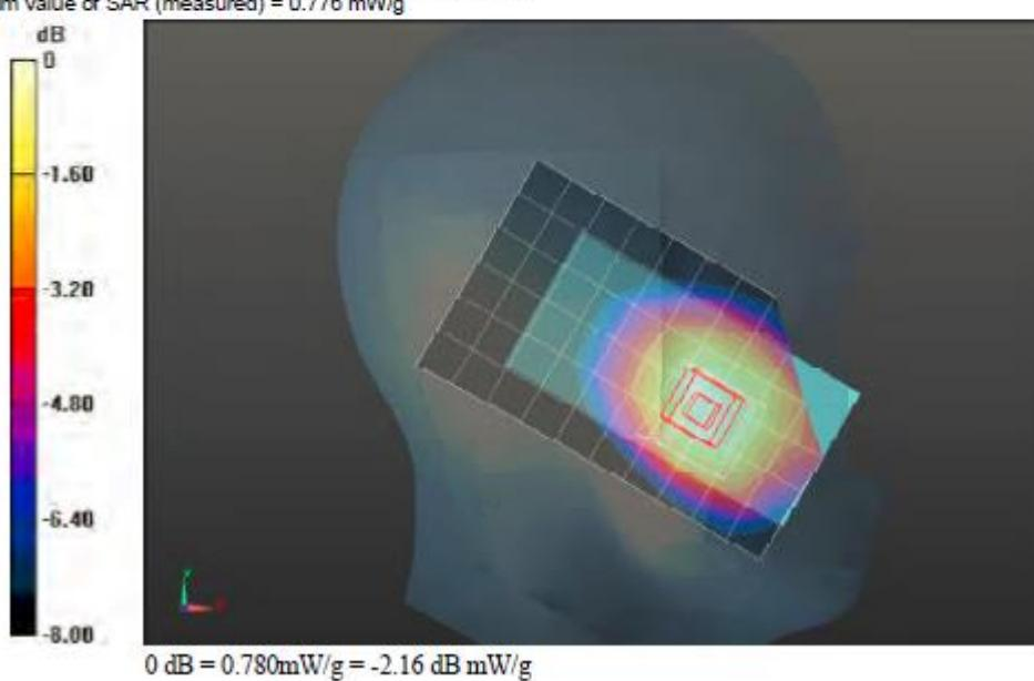
Back of EUT PCS 1900 GPRS 2Tx CH810 - UL VS Ltd
