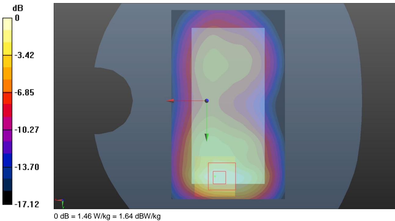
Communication System: UID 0, LTE FDD Bands - 20MHz Channel BW ; Frequency: 1732.5 MHz; Duty Cycle: 1:1
