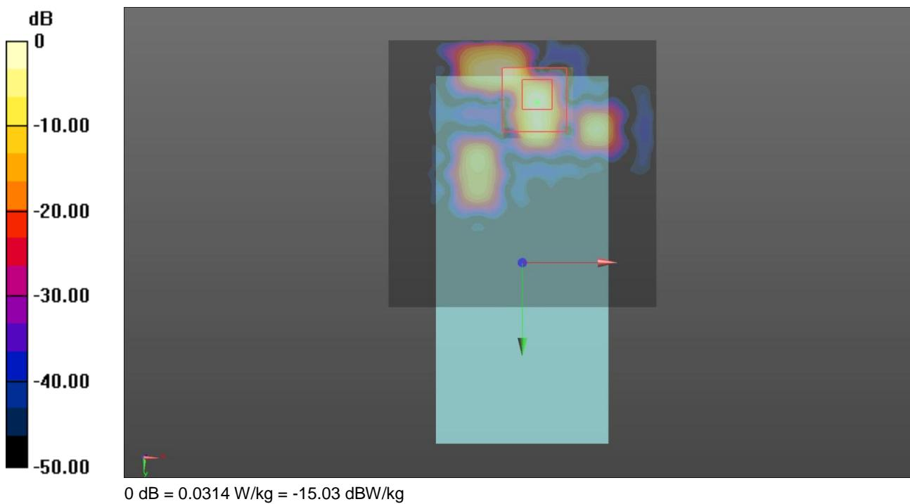
Communication System: UID 0, WLAN 802.11 (0); Frequency: 5620 MHz; Duty Cycle: 1:1
