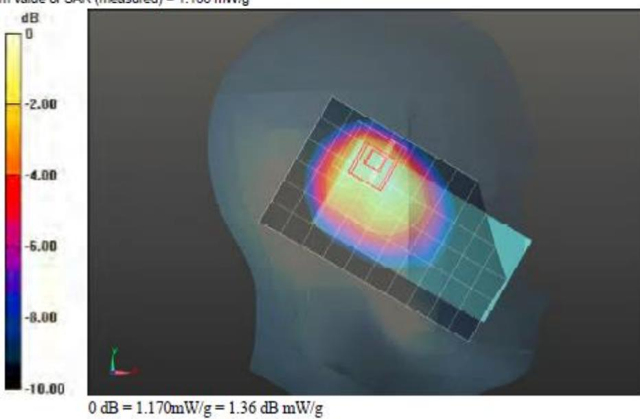
Touch Left of EUT LTE 13 CH23230 - UL VS Ltd
