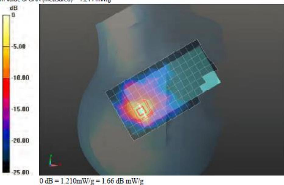
Front of EUT Wi-Fi 5.3 GHz CH64 - UL VS Ltd
