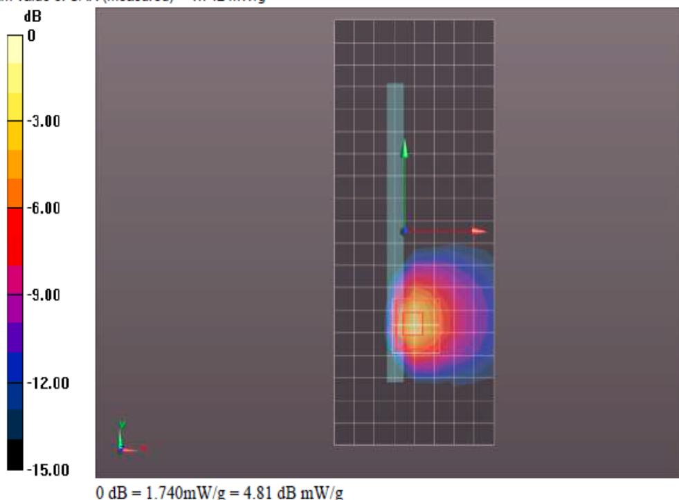
Bottom of EUT Wi-Fi 5.3GHz CH60 UL VS Ltd
