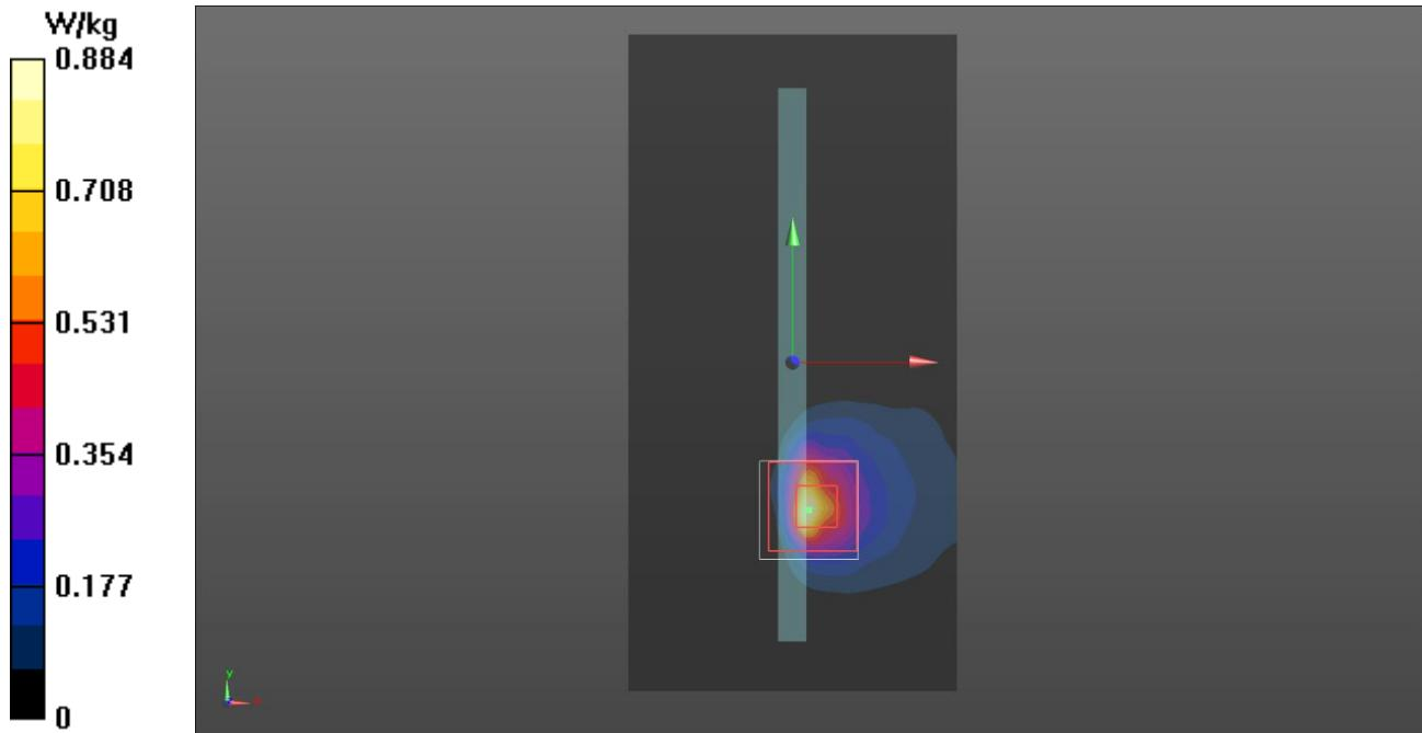
Communication System: UID 0, WLAN 802.11 (0); Frequency: 5785 MHz; Duty Cycle: 1:1
