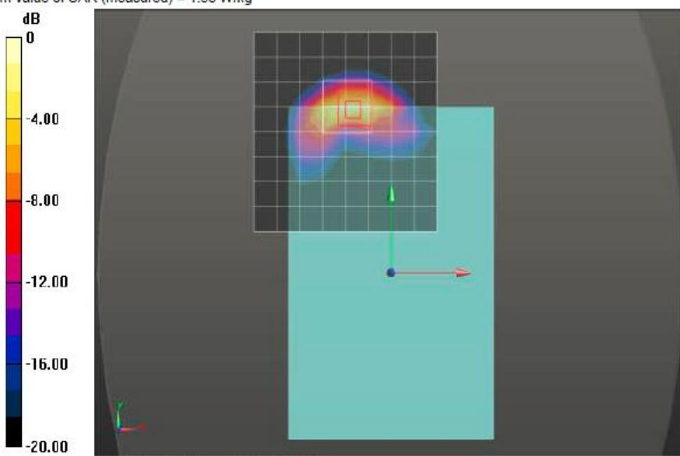
Back of EUT CDMA BC10 CH476 UL VS Ltd
