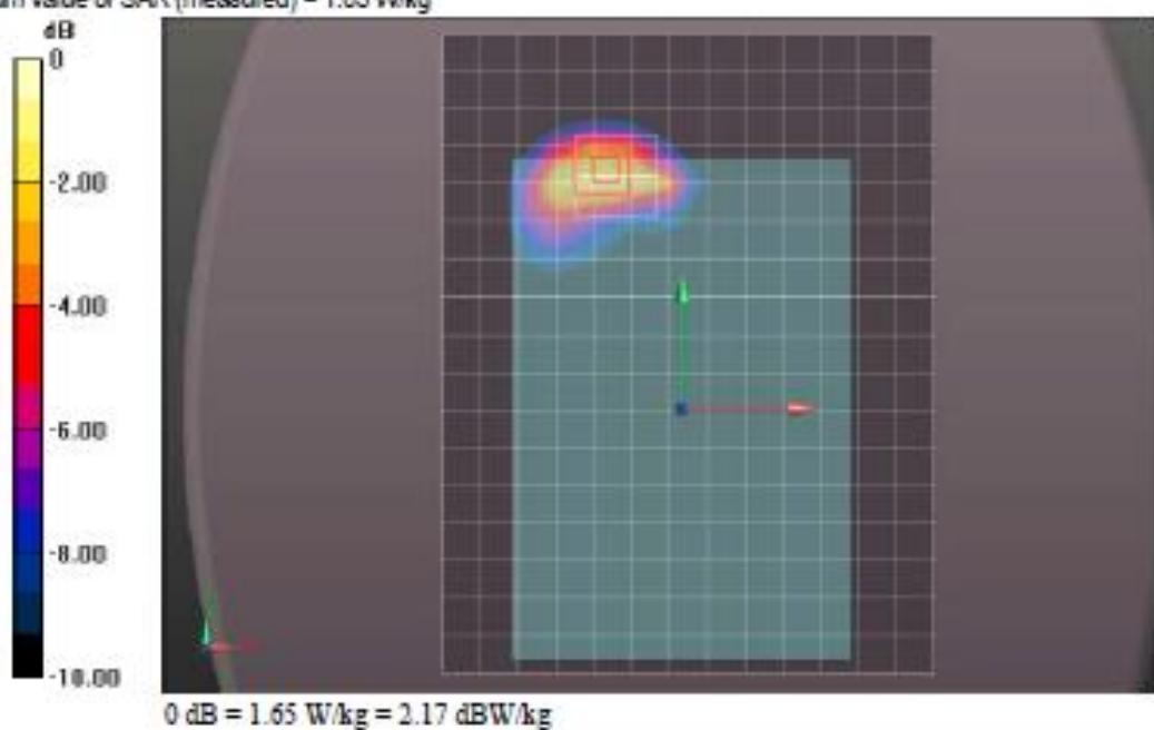
Bottom of EUT Wi-Fi 5.2GHz CH46 UL VS Ltd
