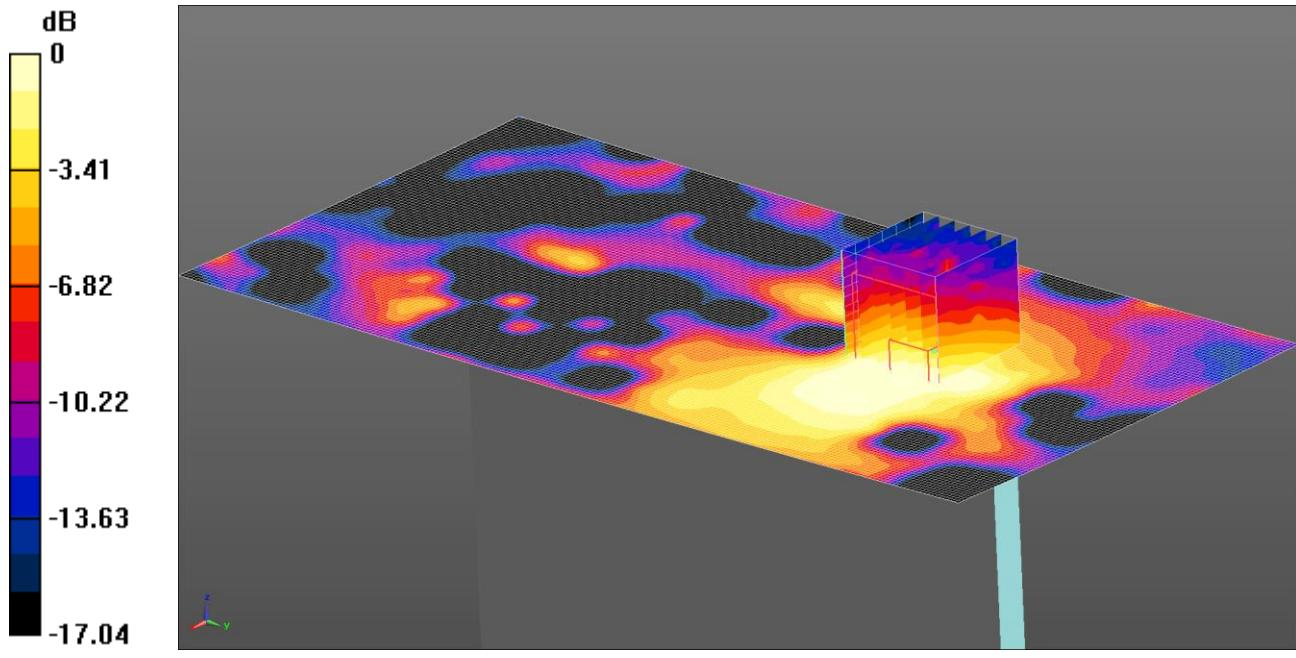
Communication System: UID 0, WLAN 802.11 (0); Frequency: 2457 MHz; Duty Cycle: 1:1
