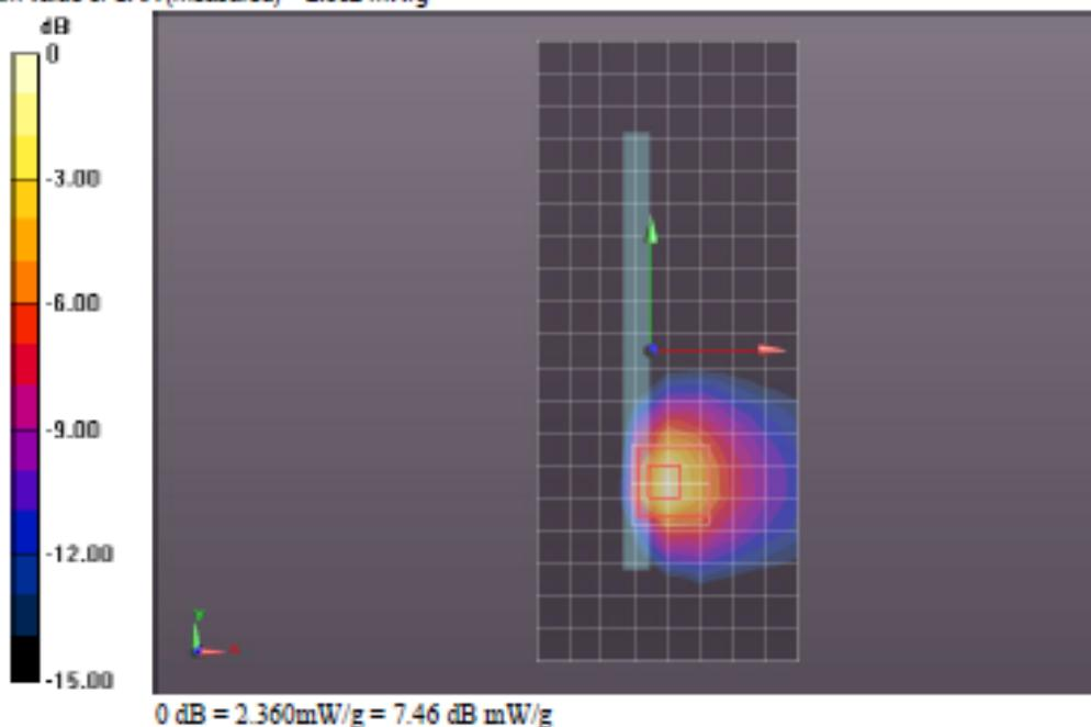
Bottom of EUT Wi-Fi 5.3GHz CH52 UL VS Ltd
