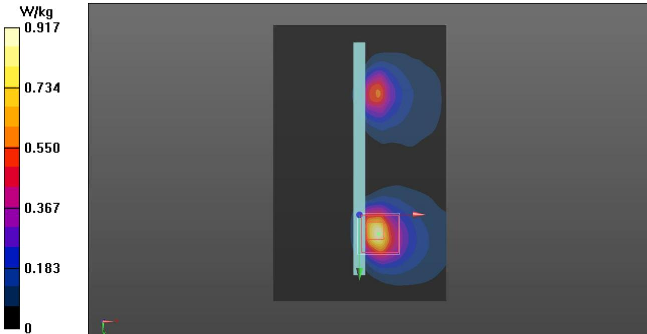
Communication System: UID 0, WLAN 802.11 (0); Frequency: 5260 MHz; Duty Cycle: 1:1
