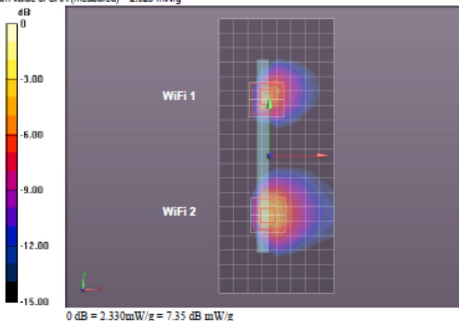
Bottom of EUT Wi-Fi 5.8GHz CH165 UL VS Ltd
