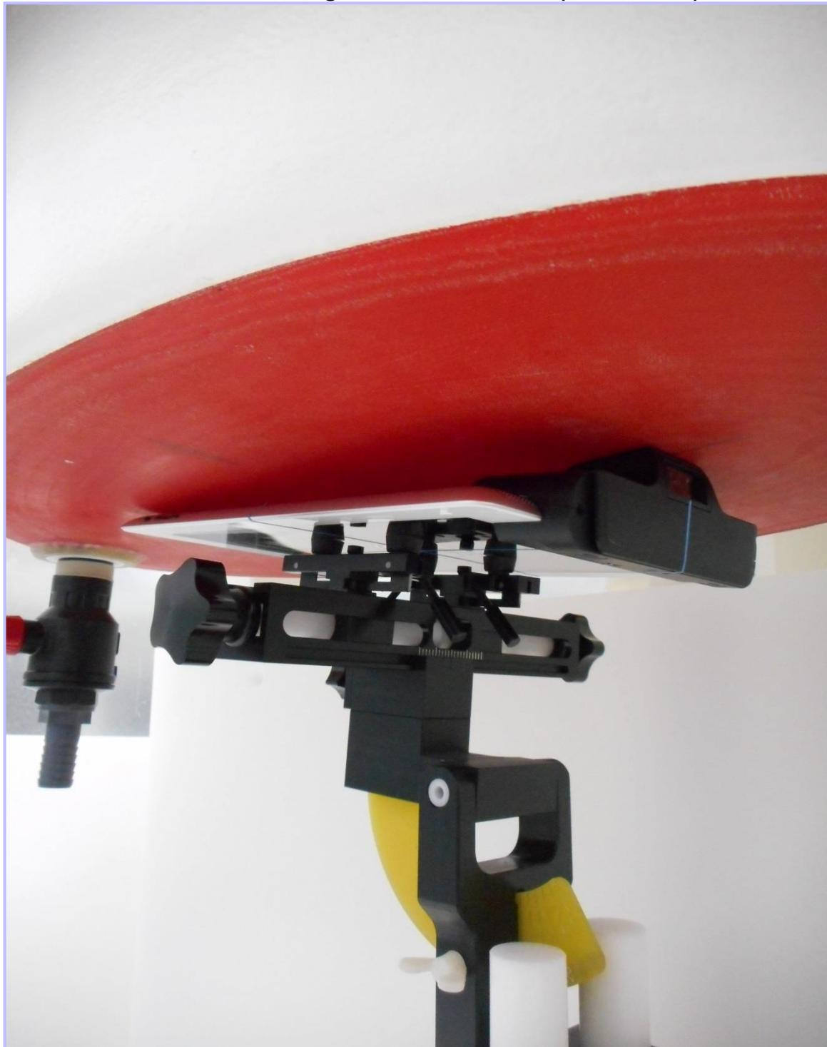
**005: Bottom of the Host EUT Facing Phantom with Sleeve (Infinea Tab 4)**
