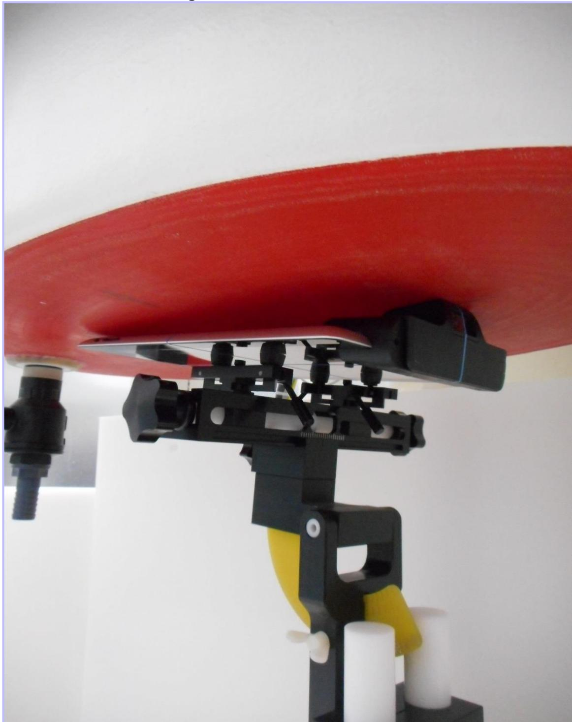
**005: Bottom of the EUT Facing Phantom with Infinea Tab Case**
