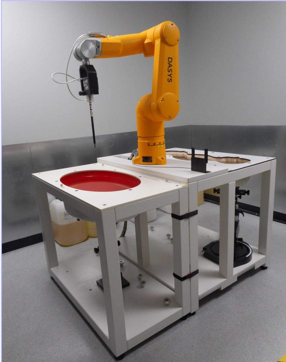
**002: Bottom of the Host EUT Facing Phantom (Standalone Configuration)**
