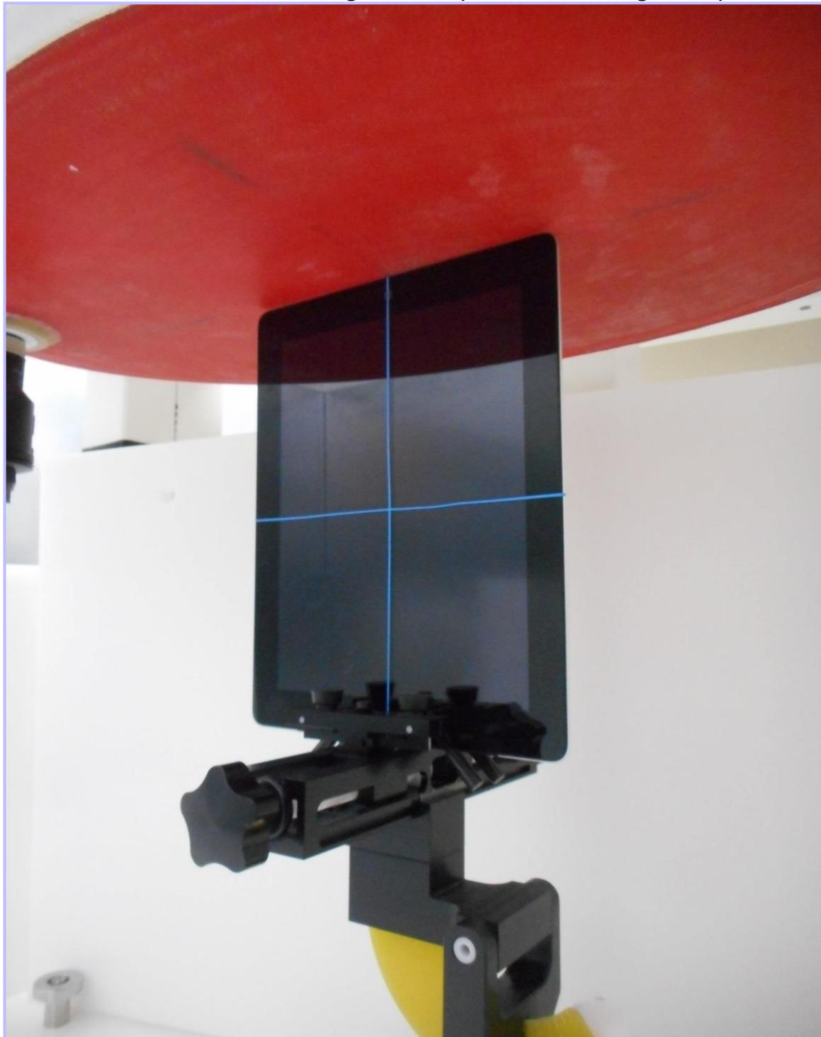
**003: Bottom of the Host EUT Facing Phantom with Sleeve (Infinea Tab 4)**
