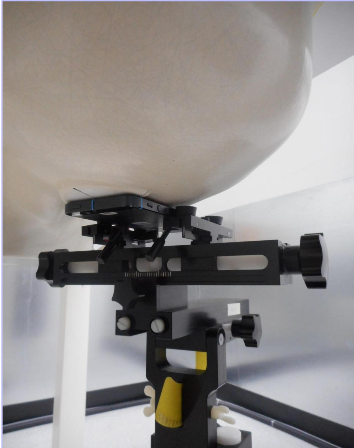
**004: Front of Host Device Facing Phantom at 10mm Separation**
