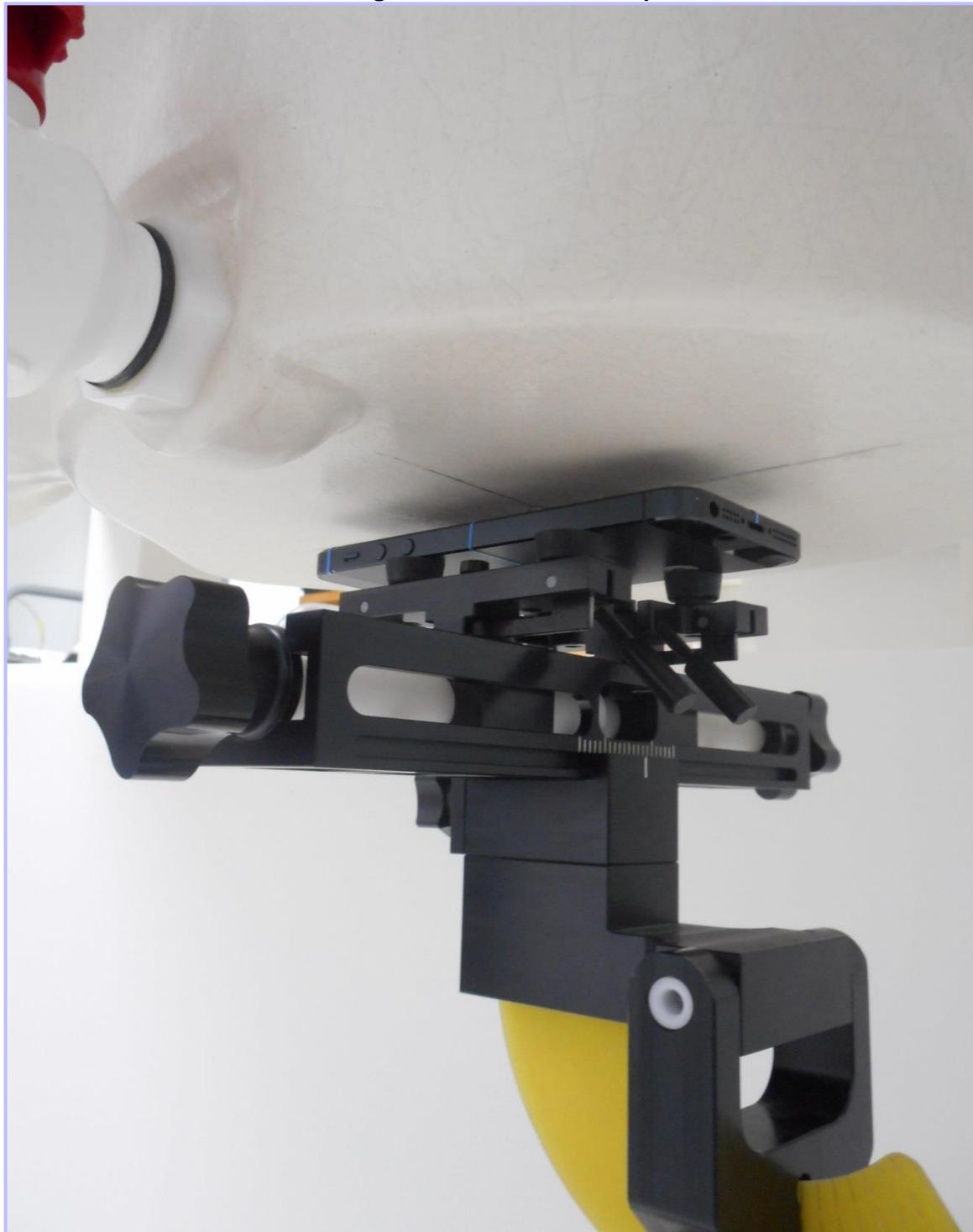
**005: Back of Host Device Facing Phantom at 10mm Separation**
