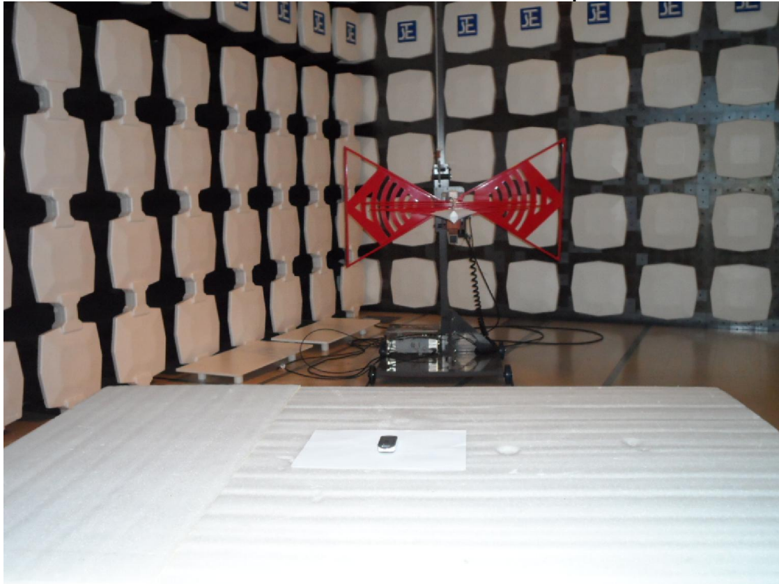
Measurement of Radiated Emission Test Set Up
