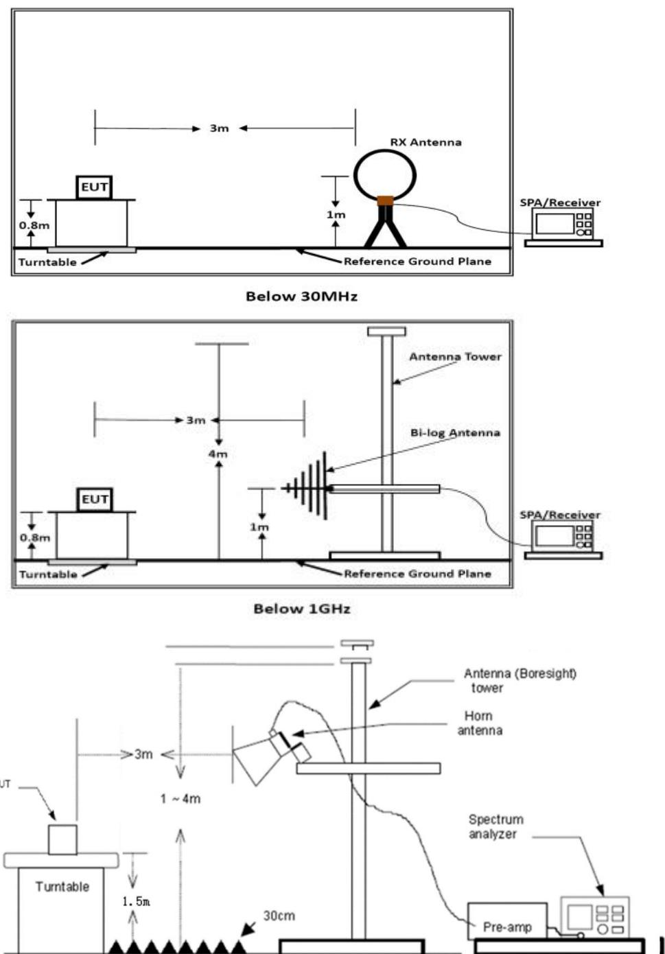
Above 18 GHz shall be extrapolated to the specified distance using an extrapolation factor of 20 dB/decade from 3m to 1m.
