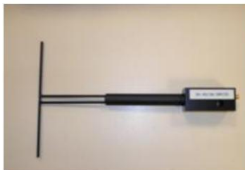
Figure 1 – Satimo COMOSAR Validation Dipole
