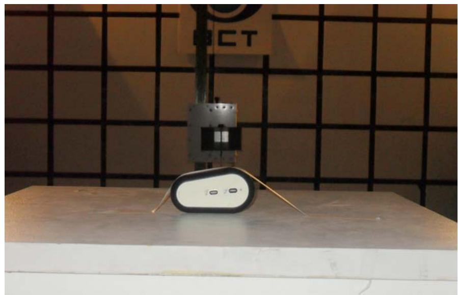
**The 3rd position is the worst case emissions of the 3 tested orthogonal positions**
