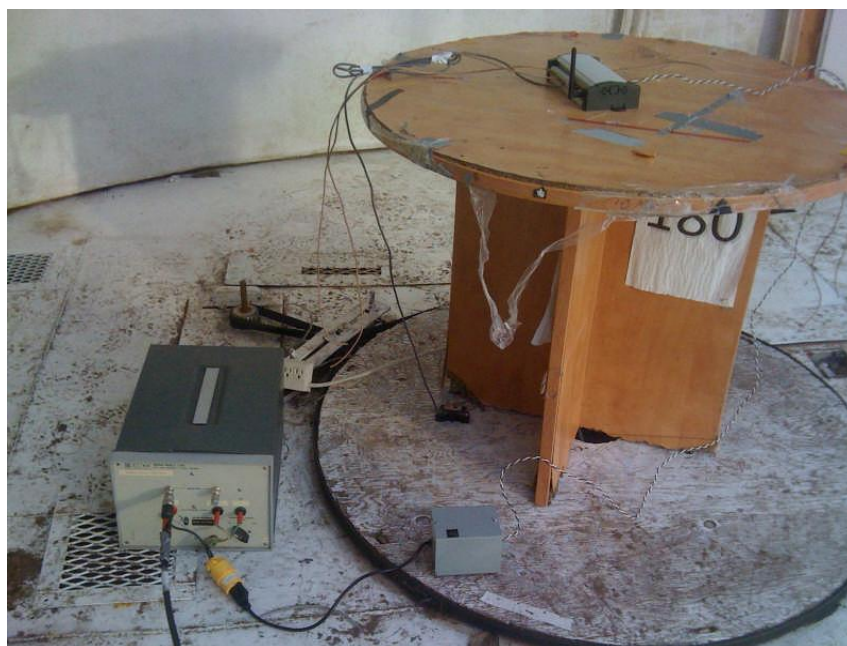
Test Setup for Conducted Emissions
