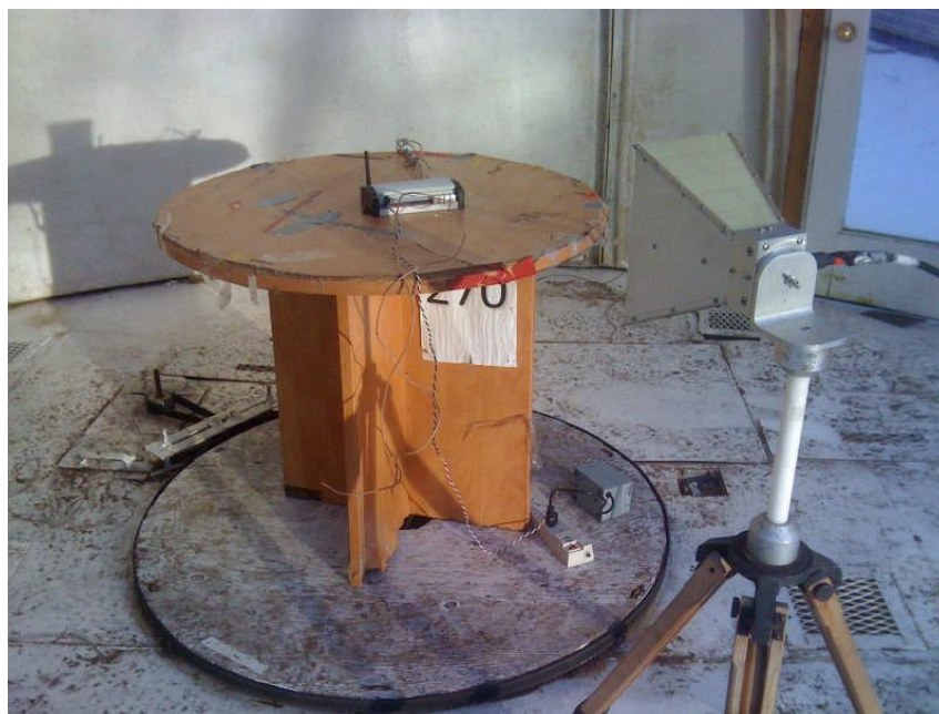
Test Setup for Radiated Emission
