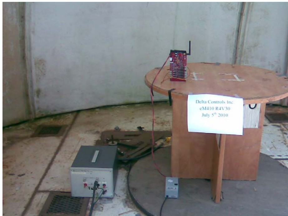
Pic 2 :Test Setup for Conducted Emissions
