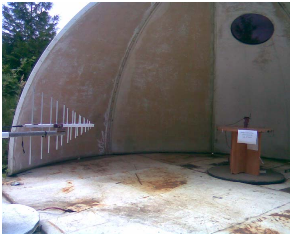
Pic 3: Test Setup for Radiated Emissions
