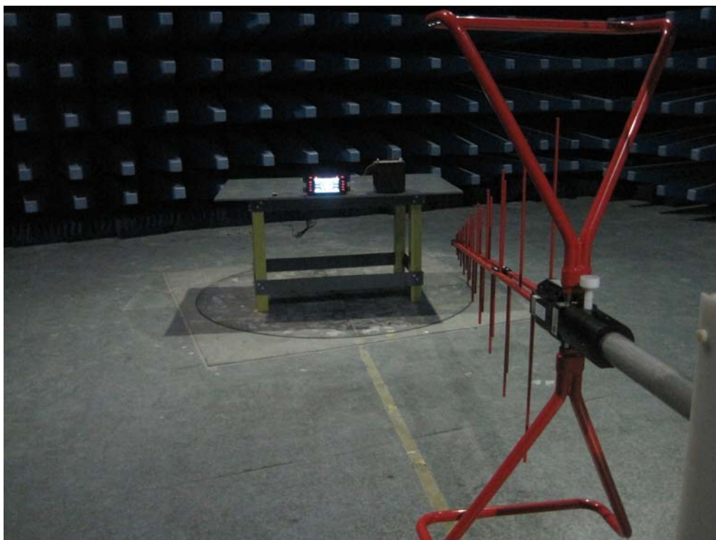
Rear View of Radiated Emission Test Setup below 1GHz
