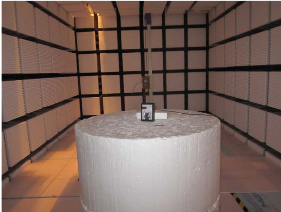
Photo of Setup for Radiated Emission
