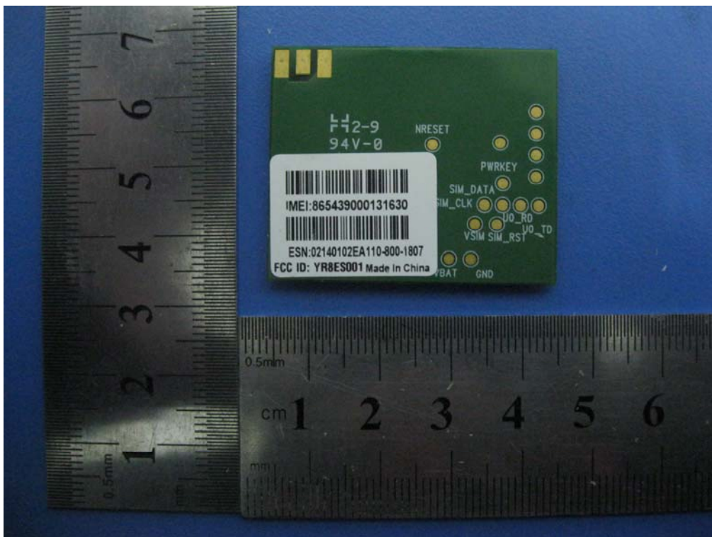
GSM Module PCB Board – Bottom View
