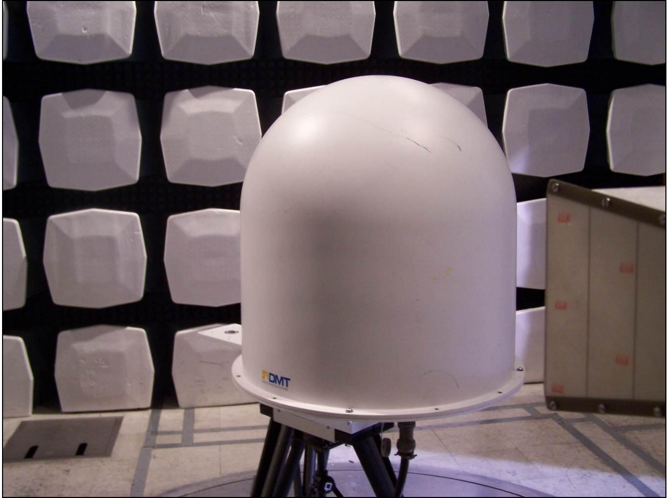
Photograph 3. Field Strength of Spurious Emissions, Test Setup
