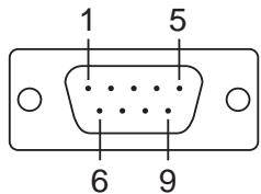
The CBL-F40M9x4-50 and CBL-F20M9x4-50 cables provide DB9 (M) connectors for each serial port, with pin assignments as follows:
