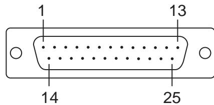
The CBL-F40M25x4-50 and CBL-F20M25x4-50 cables provide DB25 (M) connectors for each serial port, with pin assignments as follows:
