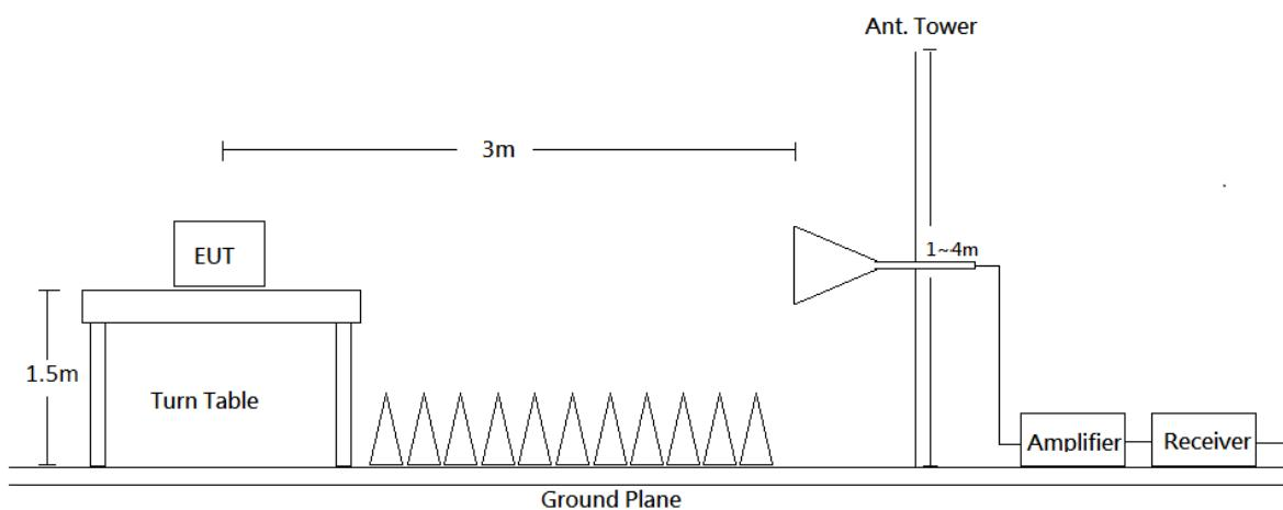
Radiated emission tests were performed in the 3 meters chamber test site, using the setup accordance with the ANSI C63.10-2013. The specification used was the FCC 15.209, and FCC 15.249 limits.
