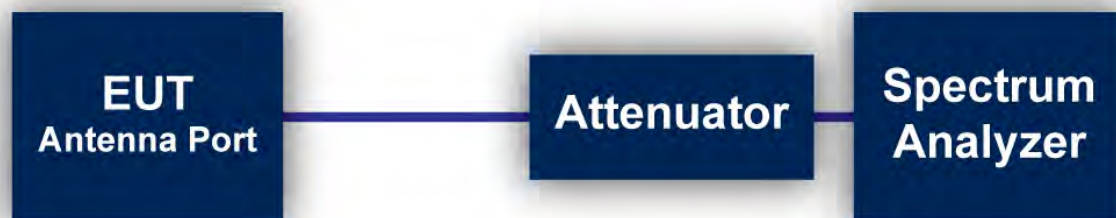
Figure 2: Direct Connection at the Antenna Port Test
